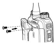
Step 3 Tighten the screws.
