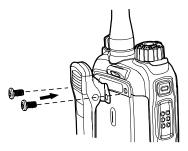
Step 3 Tighten the screws.
