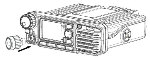
Step 2 Rotate the lock knob clockwise to fasten it.
