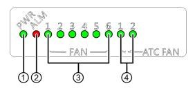
Figure 25: Indicators (LEDs) of the fan unit
