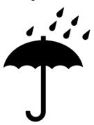
Figure 3: Safety marking "Keep dry"
