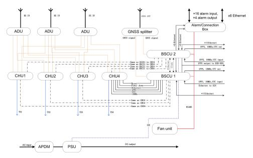
Figure 28: Internal wiring with four CHUs and external antenna coupling system
