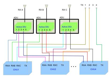
Figure 29: Antenna configuration with four CHUs and external antenna coupling system
