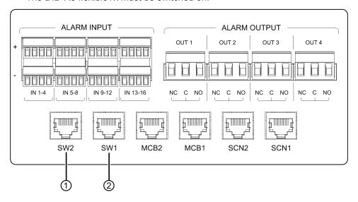
Figure 30: Connections of the service computer (local)
