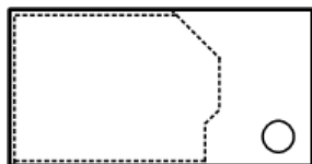
Figure 11.26 Cover of the DC voltage supply connectors - predetermined breaking pattern (rear view)
