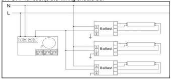
To connect Hytronik sensorDIM ballast with sensor the wiring should follow the below schematic:
