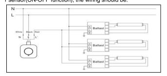
To connect several Hytronik sensorDIM ballast with 1 sensor, the wiring should follow the below schematic:
