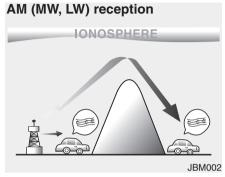
AM (MW, LW) broadcasts can be received at greater distances than FM broadcasts. This is because AM (MW, LW) radio waves are transmitted at low frequencies. These long, low frequency radio waves can follow the curvature of the earth rather than travelling straight out into the atmosphere. In addition, they curve around obstructions so that they can provide better signal coverage.
