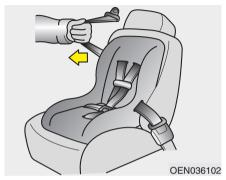
Pull the shoulder portion of the seat belt all the way out. When the shoulder portion of the seat belt is fully extended, it will shift the retractor to the "Auto Lock" (child restraint) mode.
