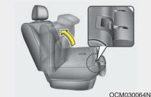
4. Pull on the seatback folding lever, then fold the seat toward the front of the vehicle. The headrest will fold forward. When you return the seatback to its upright position, always be sure it has locked into position by pushing on the top of the seatback.
