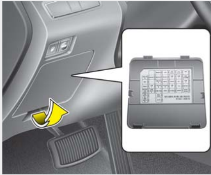
Inner panel fuse panel
