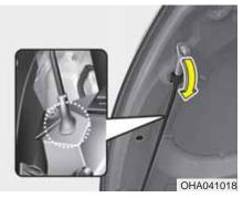
3. Pull out the support rod from the hood.4. Hold the hood open with the support rod.
