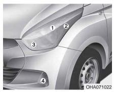
Headlight, position light, turn signal light and front fog light bulb replacement
