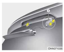
4. Disconnect the bulb electrical connector (1) by pressing the clip.
