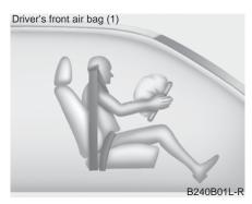
The front air bag module is located in the center of the steering wheel. When the SRSCM detects a sufficiently severe impact to the front of the vehicle, it will automatically deploy the front air bag.
