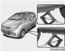
7. Place the jack at the front or rear jacking position closest to the tyre you are changing. Place the jack at the designated locations under the frame. The jacking positions are plates welded to the frame with two tabs and a raised dot to index with the jack.
