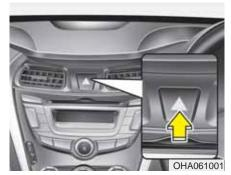
The hazard warning flasher should be used whenever you find it necessary to stop the car in a hazardous location. When you must make such an emergency stop, always pull off the road as far as possible.
