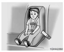
Installing a child restraint system by lap belt (on the center rear seat)
