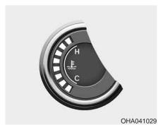
Engine coolant temperature gauge
