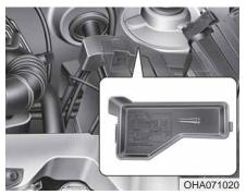
Engine compartment fuse panel Inside the fuse/relay panel covers, you can find the fuse/relay label describing fuse/relay name and capacity.
