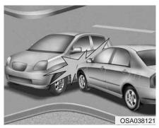
The front air bag may not inflate in side impact collisions, because occupants move to the direction of the collision, and thus in side impacts, frontal air bag deployment would not provide additional occupant protection.
