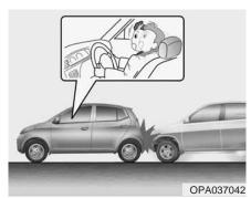
The front air bag is not designed to inflate in rear collisions, because occupants are moved backward by the force of the impact. In this case, an inflated air bag would not be able to provide any additional benefit.
