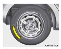
Loosen the wheel lug nuts counterclockwise one turn each, but do not remove any nut until the tyre has been raised off the ground.
