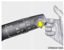
To flash the high beam headlights, pull the lever towards you. It will return to the normal (low beam) position when released. The headlight switch does not need to be on to use this flashing feature.
