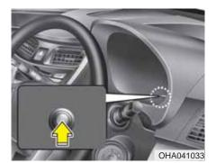
The mode will be selected by pressing the trip mode/reset button for less than 1 second.
