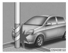
The air bag may not inflate if the vehicle collides with objects such as utility poles or trees, where the point of impact is concentrated to one area and the full force of the impact is not delivered to the sensor.
