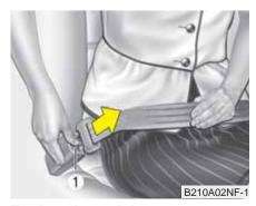
To release the seat belt: When you want to release the seat belt, press the button (1) in the locking buck-
