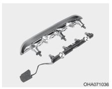
5. Pull out the bulb module from the high mounted stop light assembly by pressing in the clips (2).
