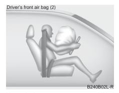
Upon deployment, tear seams molded directly into the pad covers will separate under pressure from the expansion of the air bag. Further opening of the cover then allows full inflation of the air bag.
