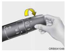
Headlight position ( ((E)) When the light switch is in the headlight position the head, tail, license and instrument panel lights are ON.
