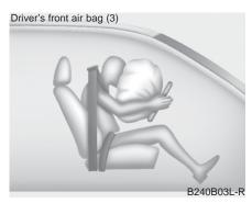
A fully inflated air bag, in combination with a properly worn seat belt, slows the driver's forward motion, reducing the risk of head and chest injury.
