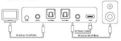
Use the BYPASS function if your TV only has ONE OPTICAL Output which is currently occupied by your AV receiver or sound bar Toggle between BYPASS and Bluetooth mode using a simple switch. No need to unplug cable. In Bypass mode, "BT5809" can be used as a decoder to convert audio between 3.5mm AUX and optical output.
