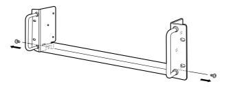
② Remove the handles from bottom bar. And turn the handles upside down, then replace the handles right side and left side.
