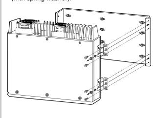
**(6)** Tighten the 3 supplied screws (M5  $\times$  12) to other side.
