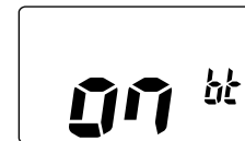
Battery voltage indication ON
