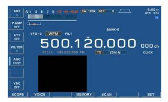
A TV tuner is built-in to the IC-R9500, and connects to the [VIDEO IN] and [VIDEO OUT] on the rear panel using a TV jumper cable to monitor the TV programs.
