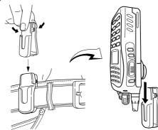
④ Once the transceiver is locked in place, it swivels as illustrated below.
