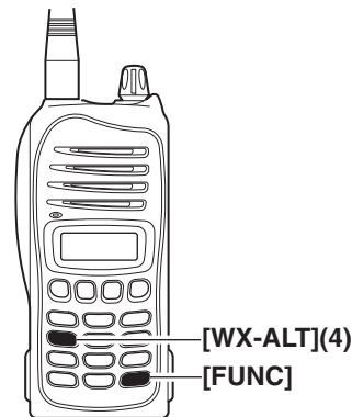
The “WX” icon appears when the weather alert is set to ON
