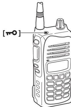
Appears while the key lock function is activated.
