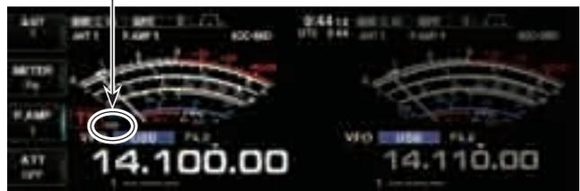
"<5W" is displayed when the power is set less than 5 W.
