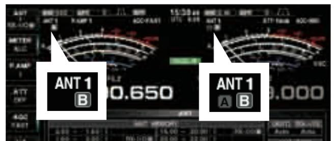
When common antenna is selected on the MAIN and SUB bands, different RX-I/O settings cannot be set. Thus, the transceiver automatically sets the RX-I/O setting of inoperating band to correct setting same as the operating side.
