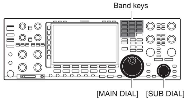
/// If the dial lock function is activated, the lock indicator lights, and [MAIN DIAL] does not function. In this case, push [LOCK] to deactivate the lock function. (see p. 4-11 for details)
