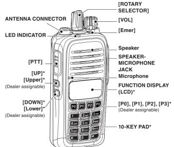
IC-F1000/F2000: Non-display type (Basic type) IC-F1000S/F2000S: Simple type (4-key type)
