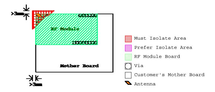
Suggestion 3: If you couldn't put RF board at one side or at the corner of mother board. You must make sure no circuit trace and grounding pad under the must isolate area, and at least reserve extra 3 mm space as safety area. Please see the drawing as below.
