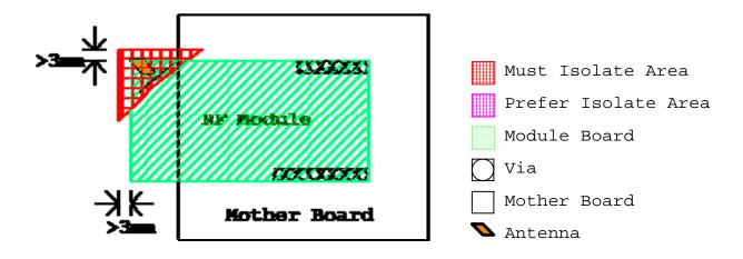
Suggestion 2: Place RF board at the corner of mother board. Make sure no trace and grounding pad under the must isolate area. Please see the drawing as below.
