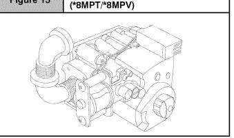
4. Gas supply line then can be run directly into opening of elbow.
