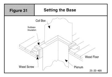
Consideration must be given to the height of the base to allow for easy installation of the condensate drain. See **Figure 32**. This subbase for combustible floors has been designed so that the height of the subbase raises the downflow coil off the floor to allow easy installation of the condensate drain
