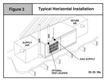
If the furnace is to be suspended from the floor joists in a crawl space or the rafters in an attic, it is necessary to use steel pipe straps or an angle iron frame to attach the furnace. These straps should be attached to the furnace bottom side with sheet metal screws and to the rafters or joists with bolts. The preferred method is to use an angle iron frame bolted to the rafters or joists.
