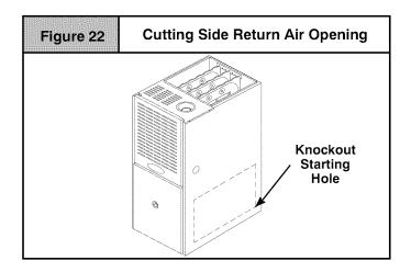
Bottom returns can be made by removing the knockout panel in the furnace base. Do **NOT** remove knock-out except for a bottom return.
