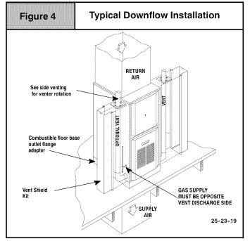
**Downflow Venting:** The combustion venter **MUST** be rotated to vent out the side for all downflow installations, (see **Figure 4**). Bottom venting is not permitted. See "**Side venting**" for instructions to rotate the vent to the side. In addition to rotating the vent to the side, a **Vent Pipe Shield** (NAHA002VC) is required to shield the hot vent pipe.
