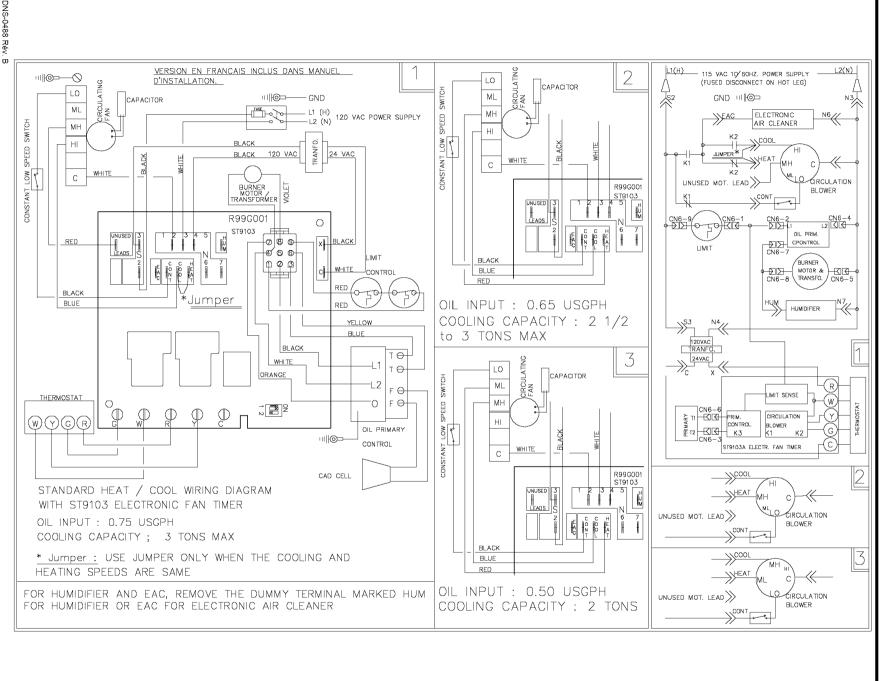
FIGURE # 4 Wiring diagram, NOMF105D12A, Beckett burner Rév
