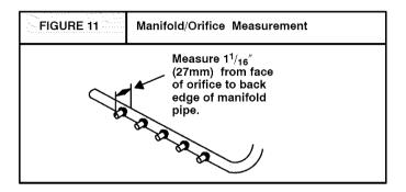
Install the correct orifices. Gauge the size of the orifices with a new twist drill bit of the correct size.
