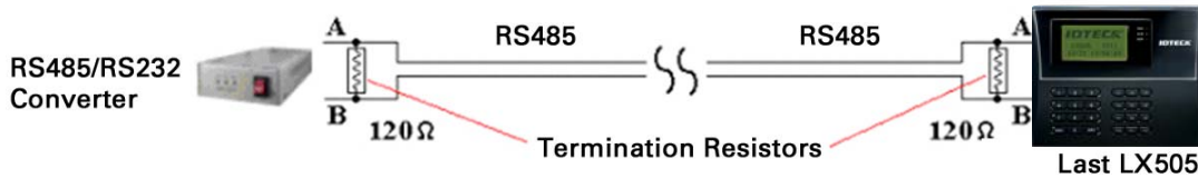
Figure: Termination resistors for 2 wire RS485 communication system
