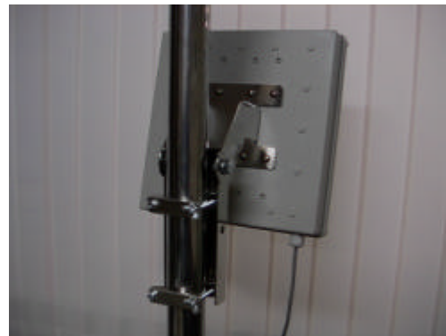
(4) Install mounting bracket to the pole then adjust the angle of the reader
