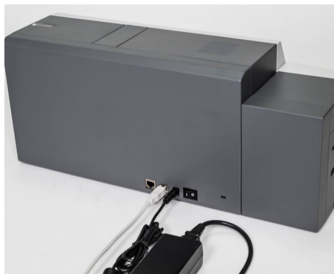
Figure 9 CP55 Dual Connection of power and USB cable
