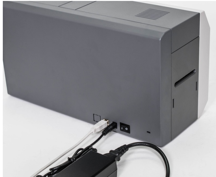
Figure 8 CP55 Connection of power and USB cable
