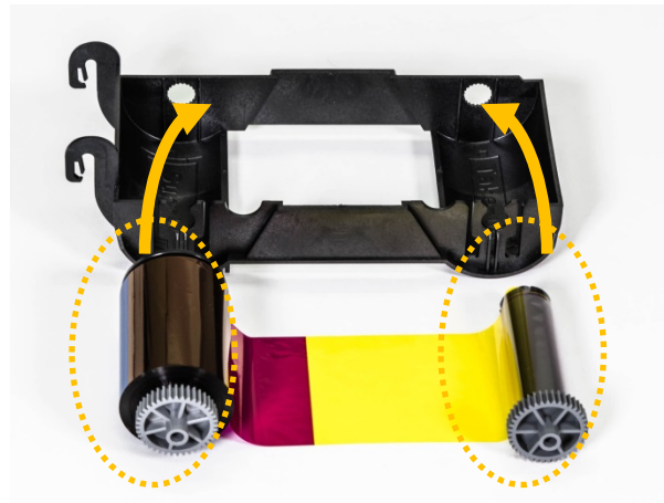
Figure 15 Loading the ribbon 1
