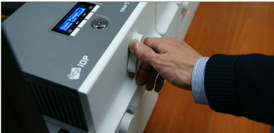
Figure 20 Ribbon / film cartridge unlocking
