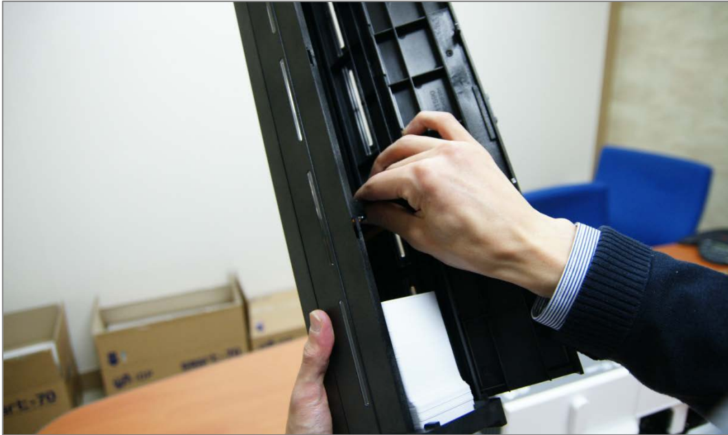
Figure 39 Putting down the card cartridge's weight
