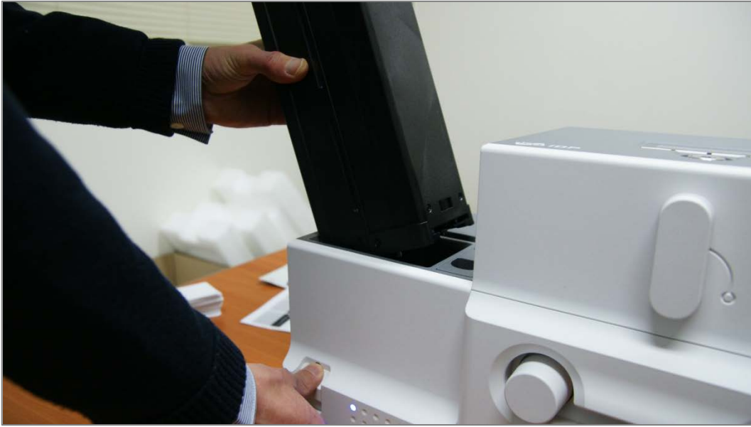
Figure 33 Card cartridge release from Input Hopper
