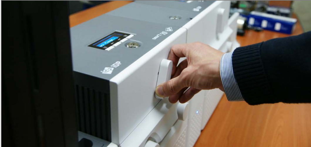
Figure 27 Ribbon / film cartridge locking
