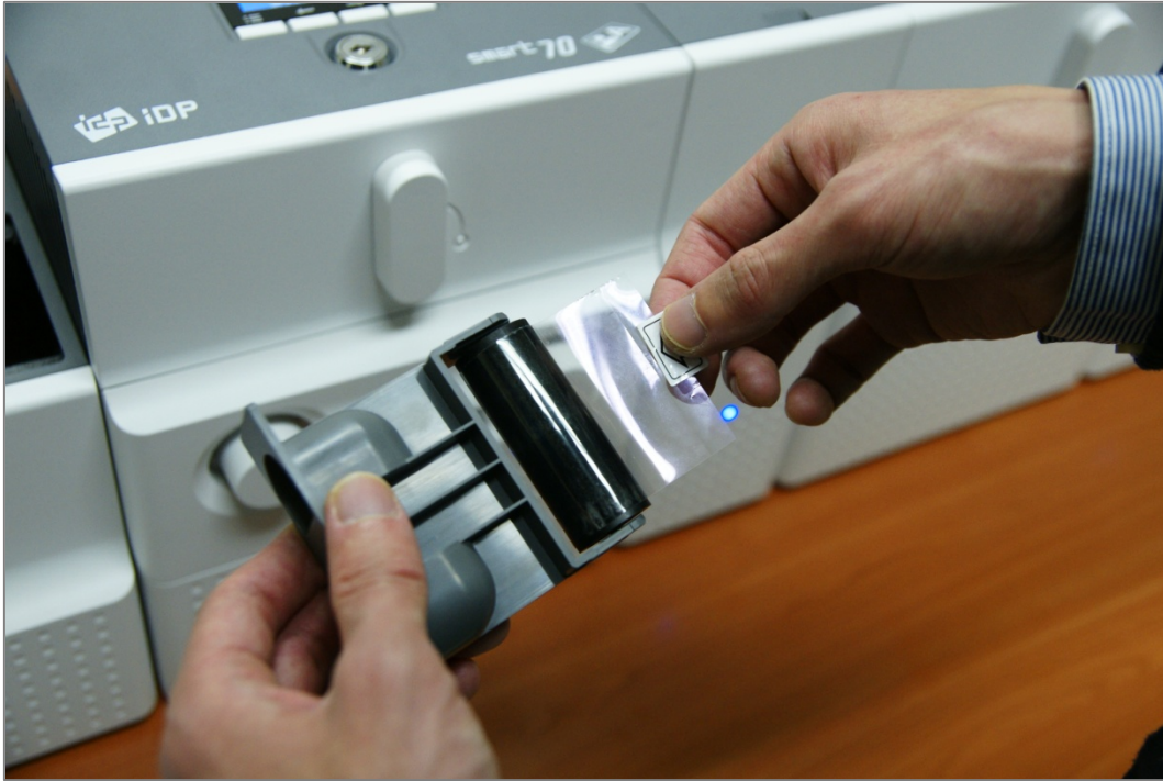
Figure 31 Removal of new disposable cleaning roller protector
