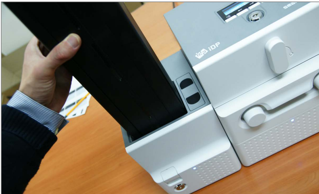
Figure 40 Loading card cartridge into Input Hopper
