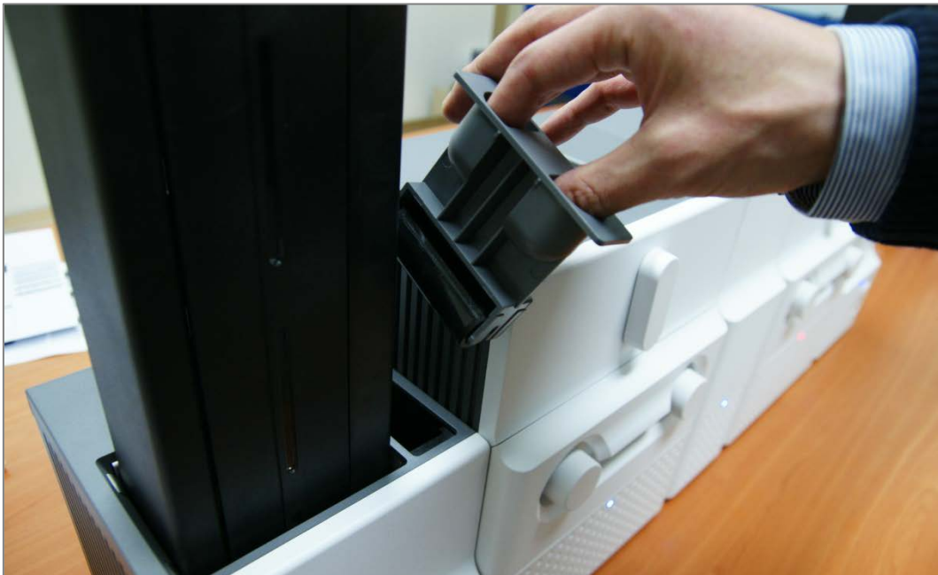
Figure 32 Installation of disposable cleaning roller holder
