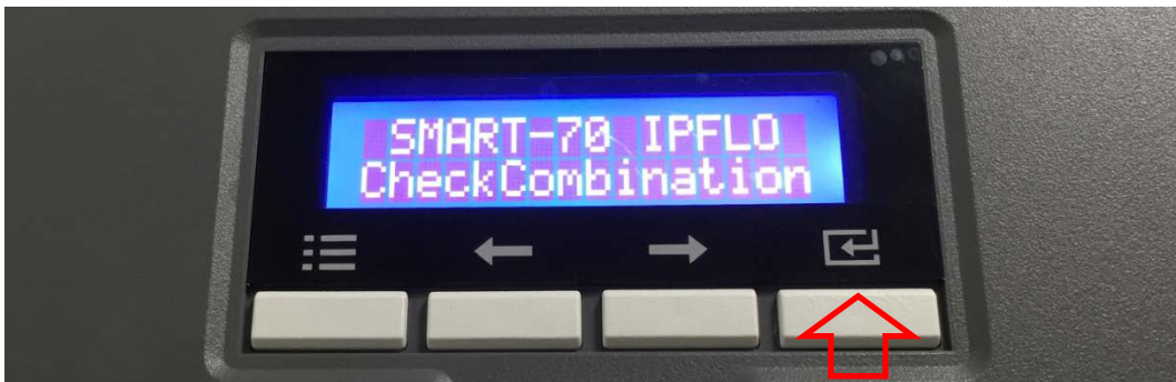
Figure 43 Modules combination checking
