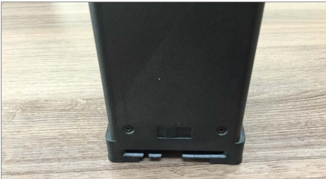
Figure 34 Cards thickness adjustment
