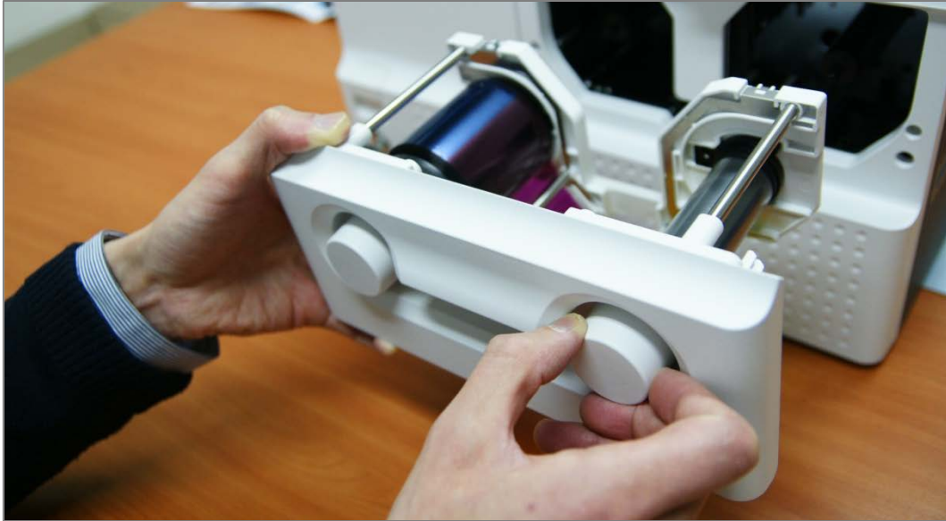
Figure 25 Print ribbon / laminating film alignment
