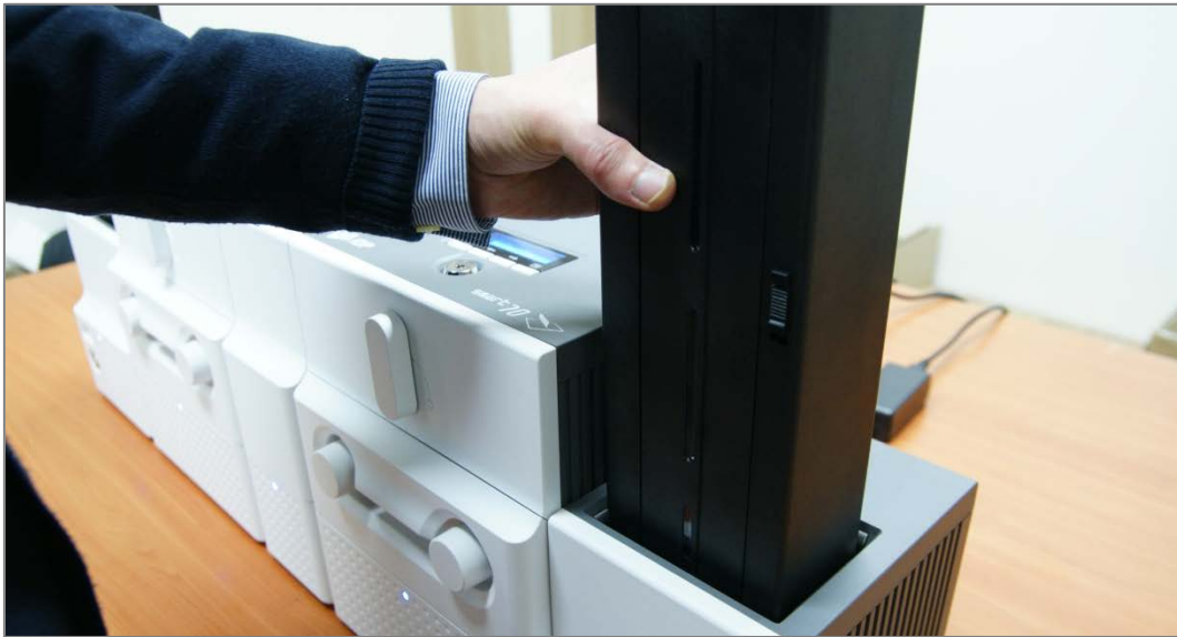
Figure 41 Loading card cartridge into Output Hopper
