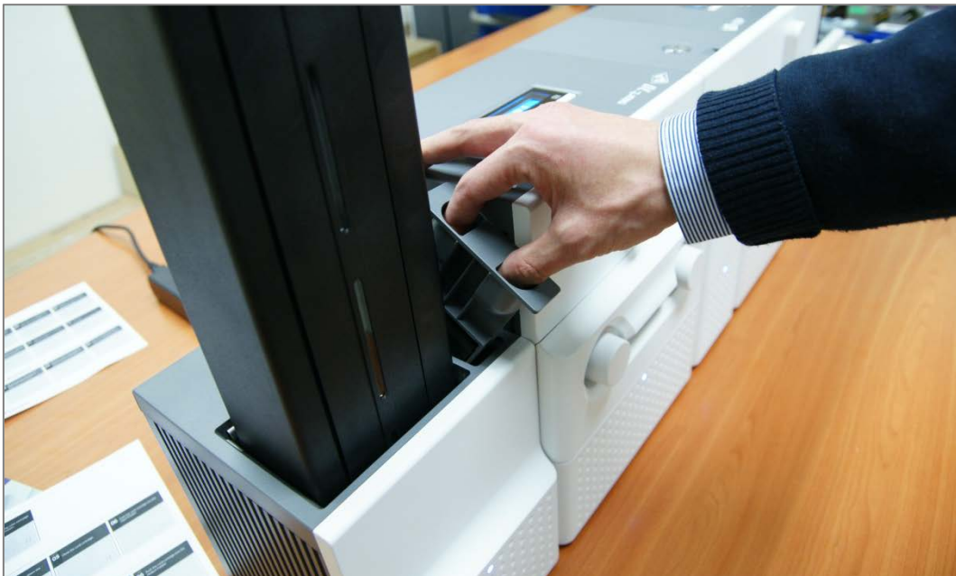
Figure 28 Detachment of disposable cleaning roller holder
