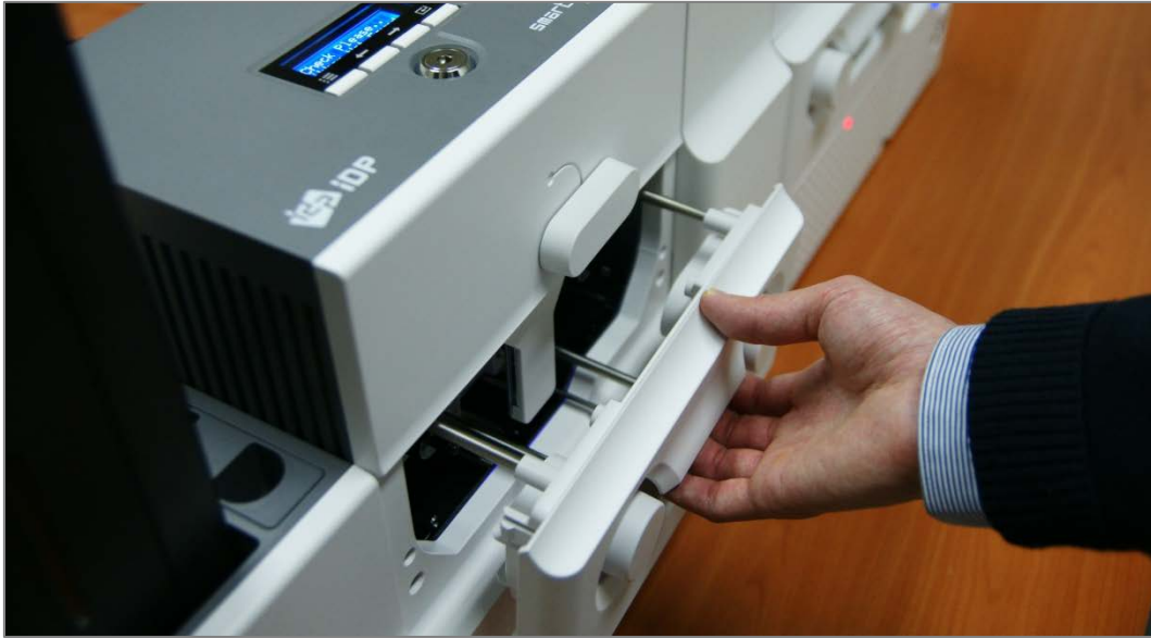
Figure 21 Pulling out ribbon / film cartridge
