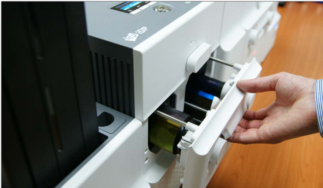
Figure 26 Ribbon / film cartridge insertion
