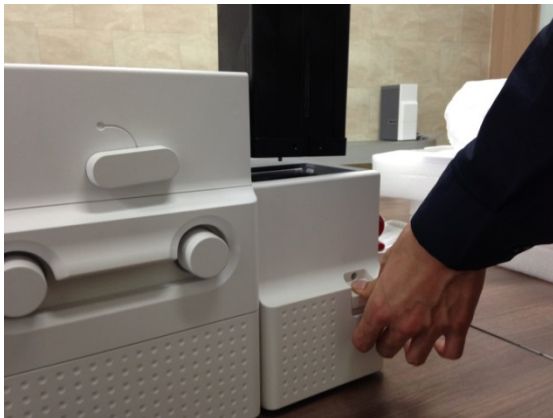
Figure 129 Card jam in Output Hopper 4
