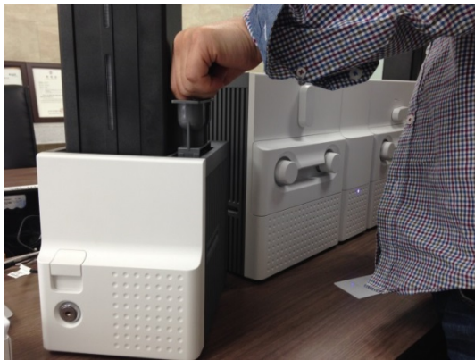
Figure 132 Input Hopper cleaning 2
