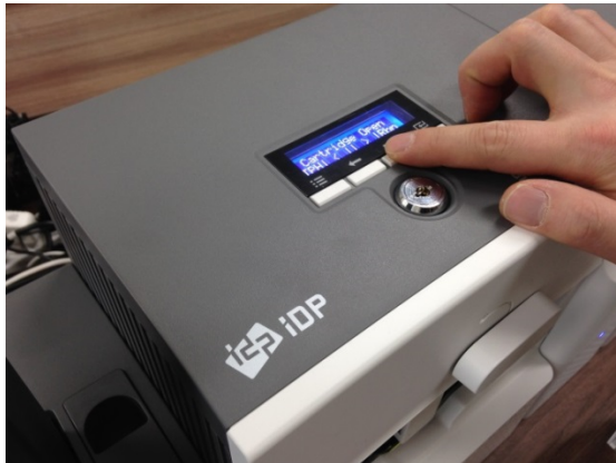
Figure 124 Card jam in Laminator 4
