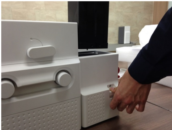
Figure 144 Output Hopper cleaning 2
