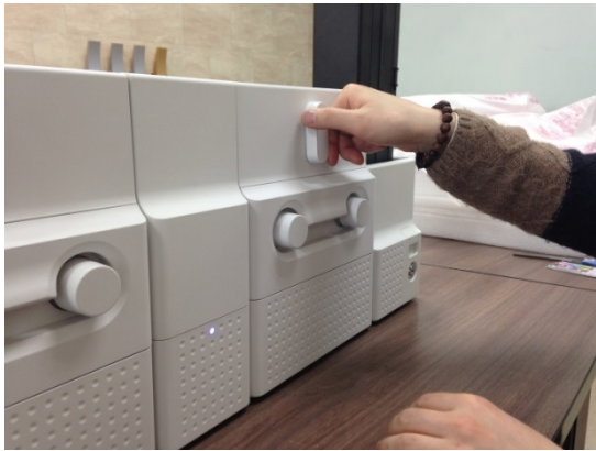
Figure 152 Laminator Head replacement 1
