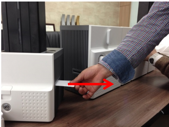
Figure 108 Card jam in Input Hopper 2
