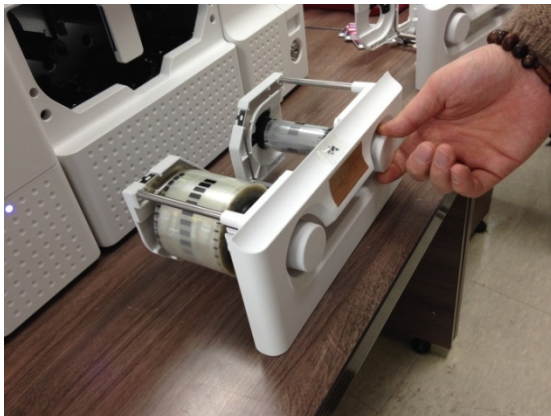
Figure 127 Card jam in Output Hopper 2
