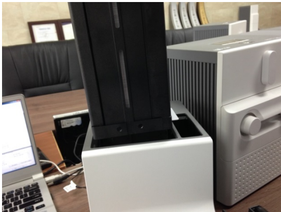
Figure 111 Card jam in Input Hopper 5
