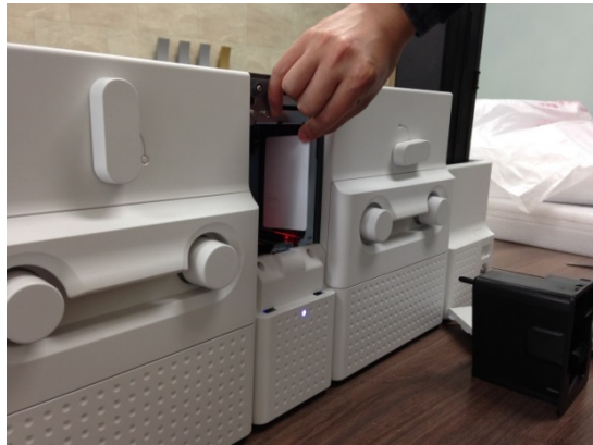
Figure 120 Card jam in Flipper 4
