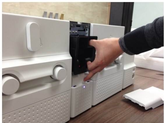
Figure 118 Card jam in Flipper 2
