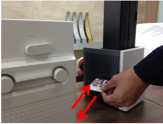
Figure 128 Card jam in Output Hopper 3
