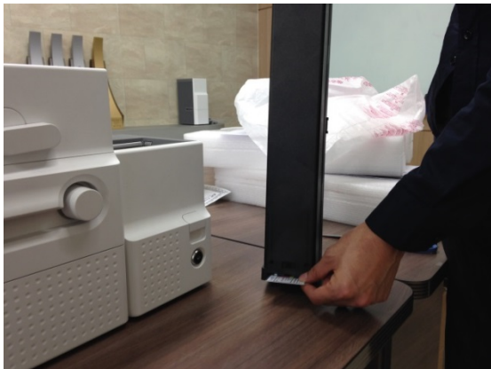
Figure 130 Card jam in Output Hopper 5
