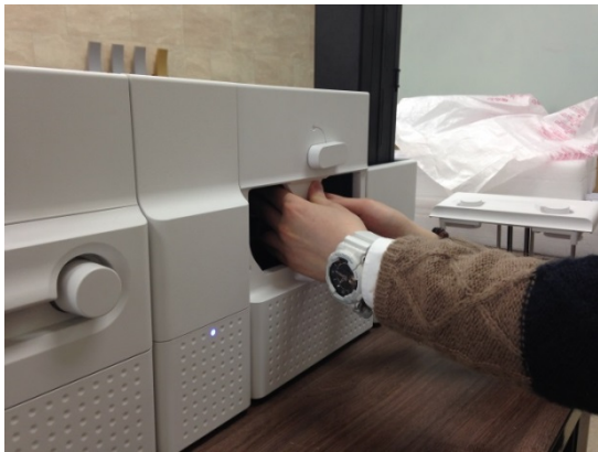
Figure 154 Laminator Head replacement 3
