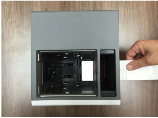
Figure 134 Input Hopper cleaning 4
