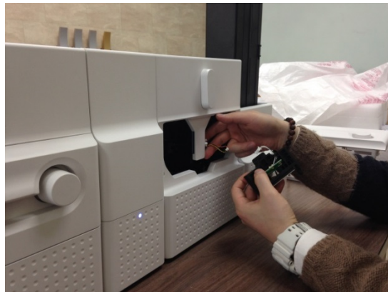
Figure 156 Laminator Head replacement 5
