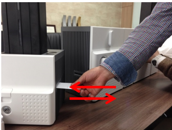
Figure 109 Card jam in Input Hopper 3
