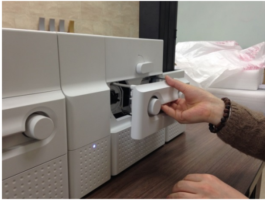
Figure 153 Laminator Head replacement 2
