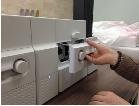
Figure 122 Card jam in Laminator 2
