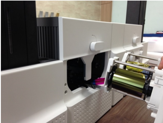
Figure 114 Card jam in Printer 3
