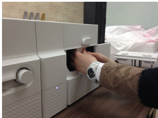
Figure 157 Laminator Head replacement 6
