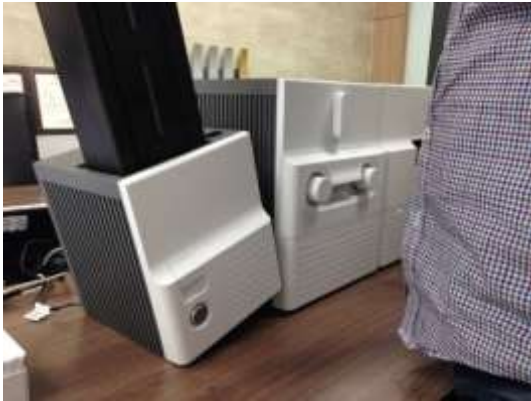
Figure 131 Input Hopper cleaning 1
