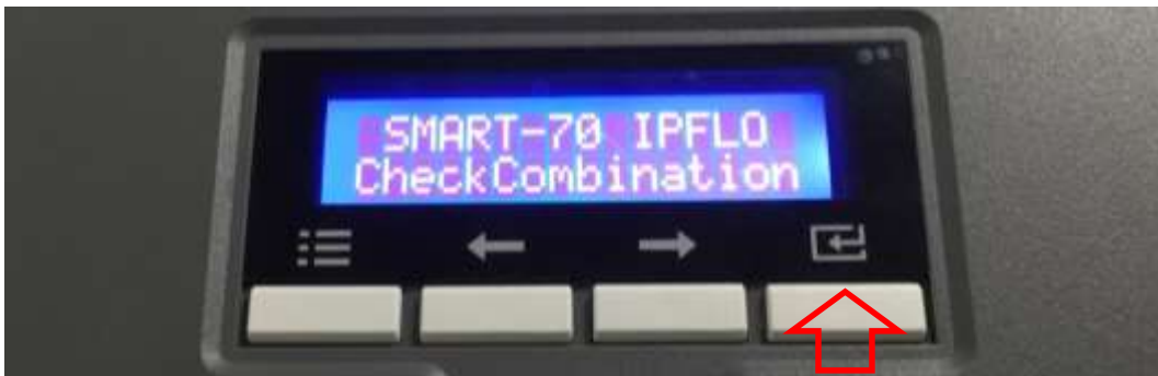
Figure 43 Modules combination checking
