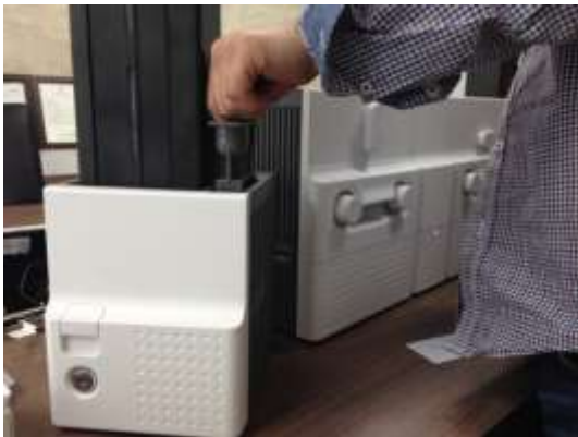
Figure 132 Input Hopper cleaning 2
