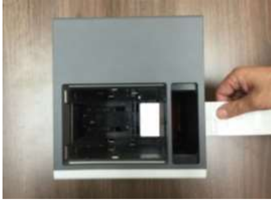
Figure 134 Input Hopper cleaning 4
