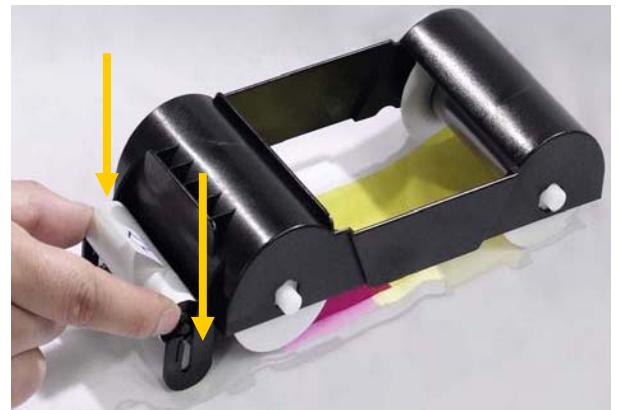
<Figure 9> Install the cleaning roller
