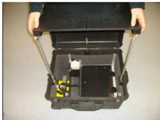
Fig. 3-8 – Fixing the worktable
