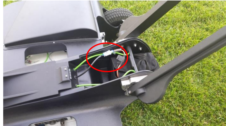
Fig. 4.11 – Connecting the main battery (male/female connectors are in the red circle)
