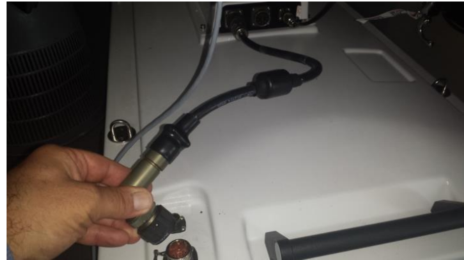
Fig. 4.7 – Connecting antenna cable
