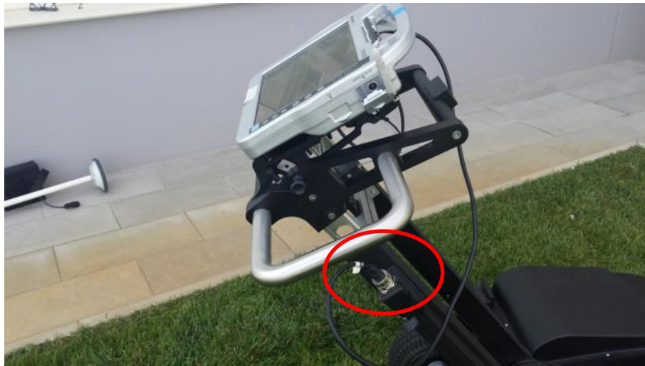
Fig. 4.12 – connecting the laptop through the LAN cable (red circle)
