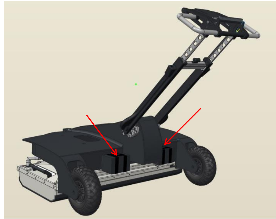
Fig. 3.9 – The position of the batteries powering the electric motor to operate the system (red arrows)
