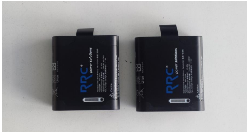
Fig. 14 – Li-ion batteries for C-Thru
