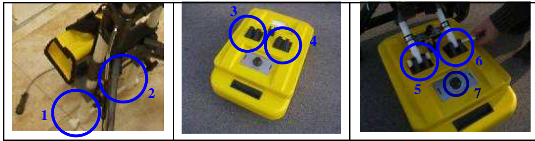
Fig. 4.5 – Fixing the antenna box
