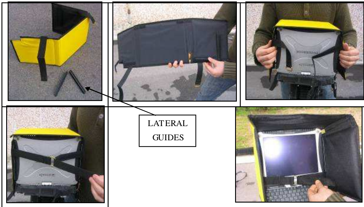
Fig. 4.9 – Assembling the sunshade
