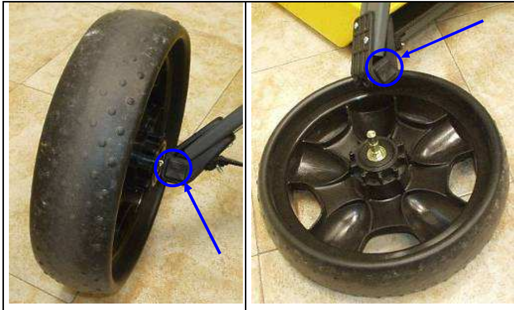
Fig. 4.12 – Removing the trolley wheels
