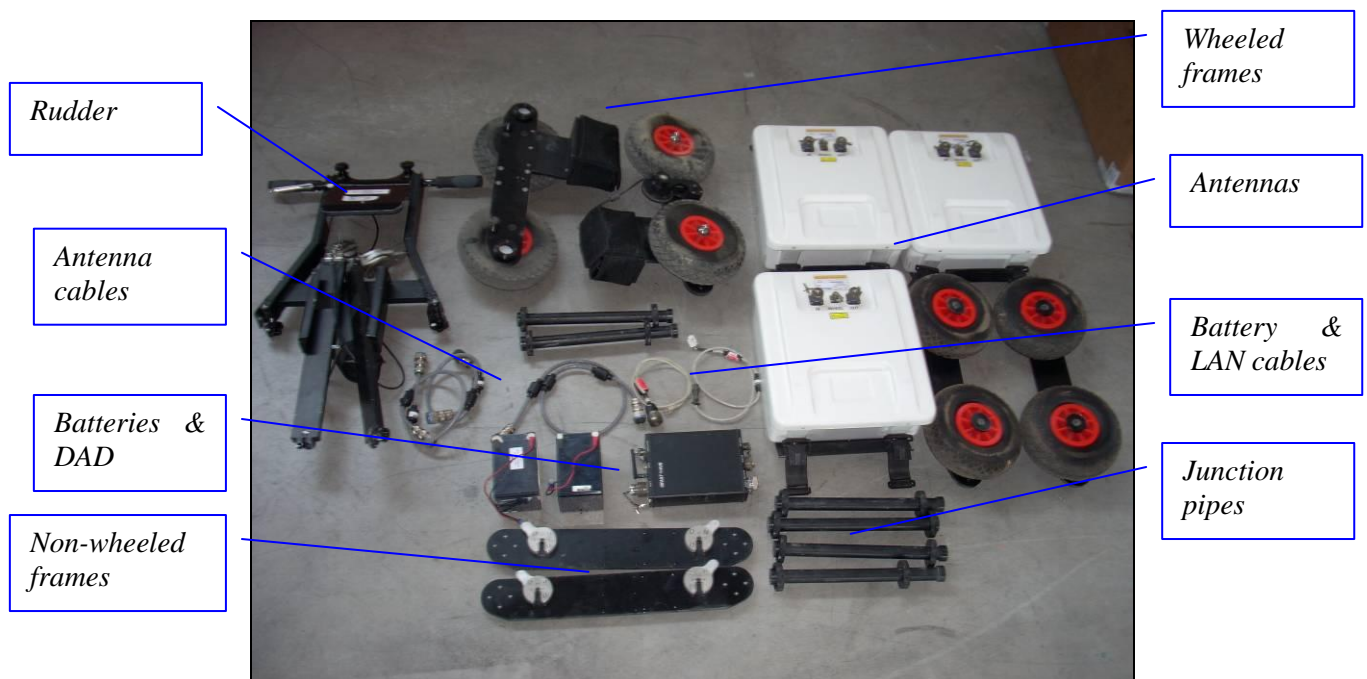
Fig. 1-21 - Equipment provided for the three antennas configuration
