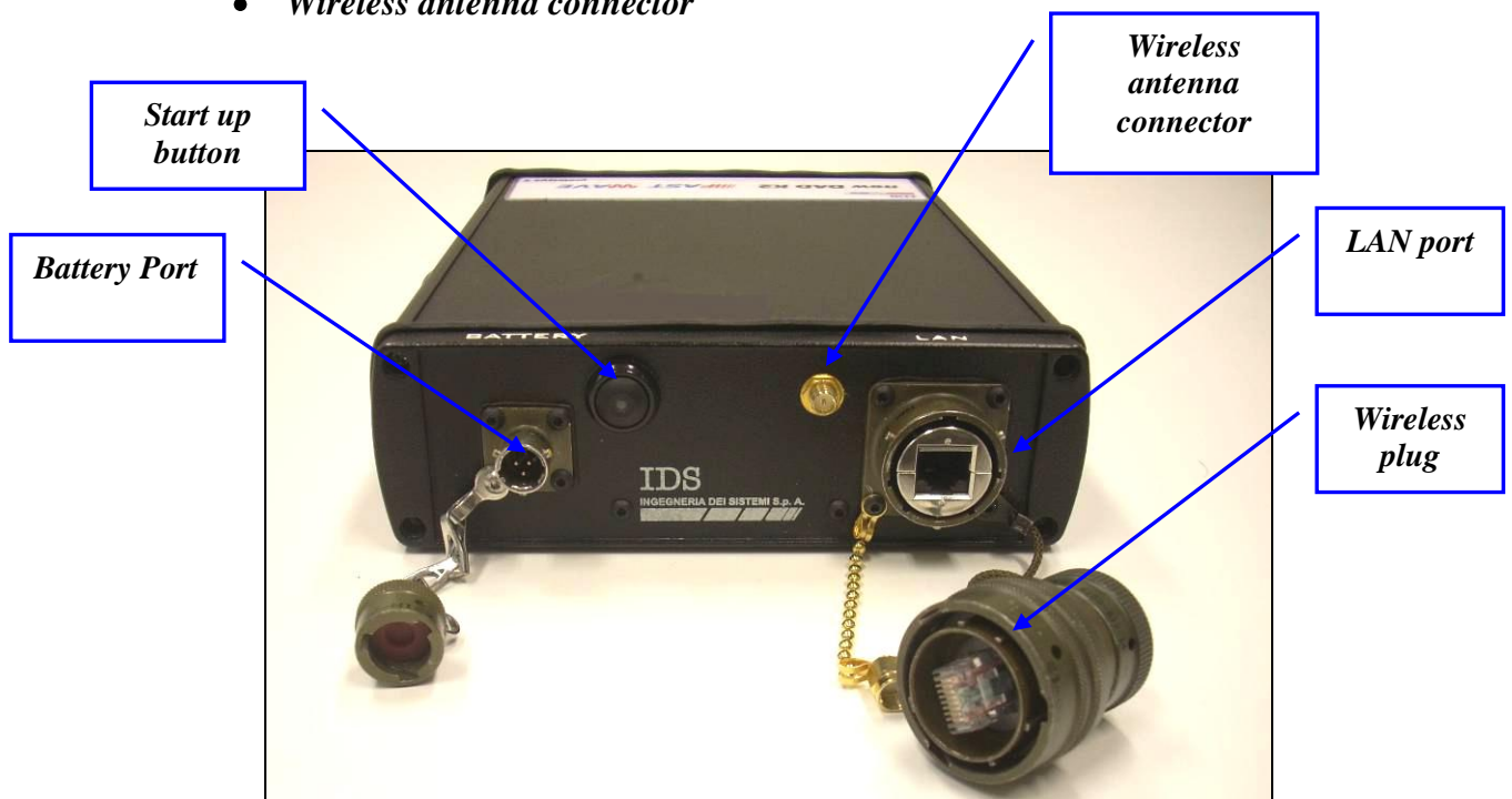
Fig. 2-1 – DAD side Fast Wave with Battery Port, Lan Port and wireless connector
