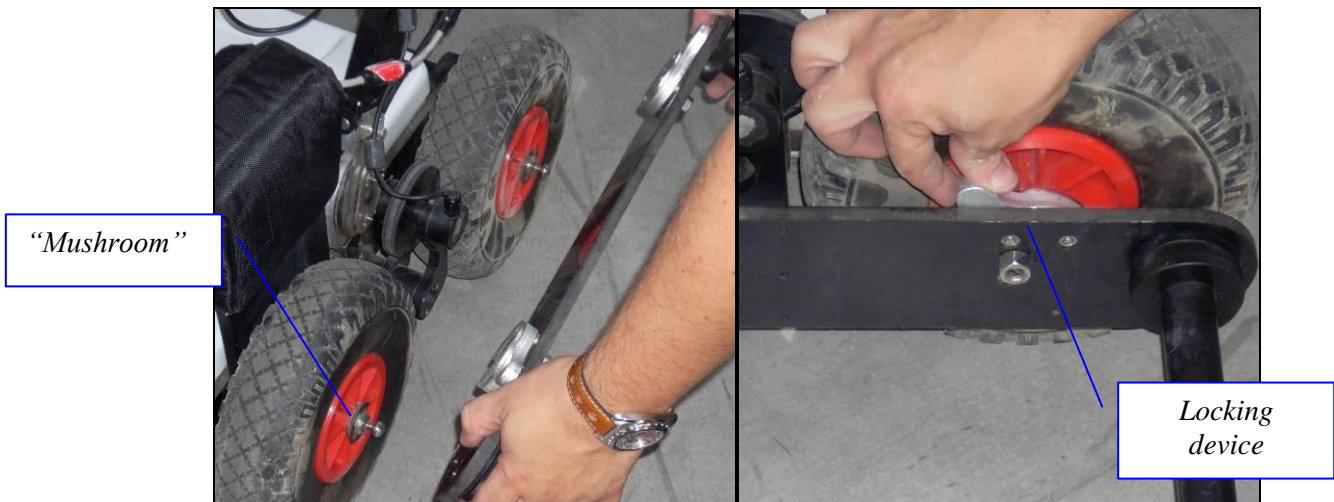
Fig. 1-24 – Main frame “mushrooms” & locking device
