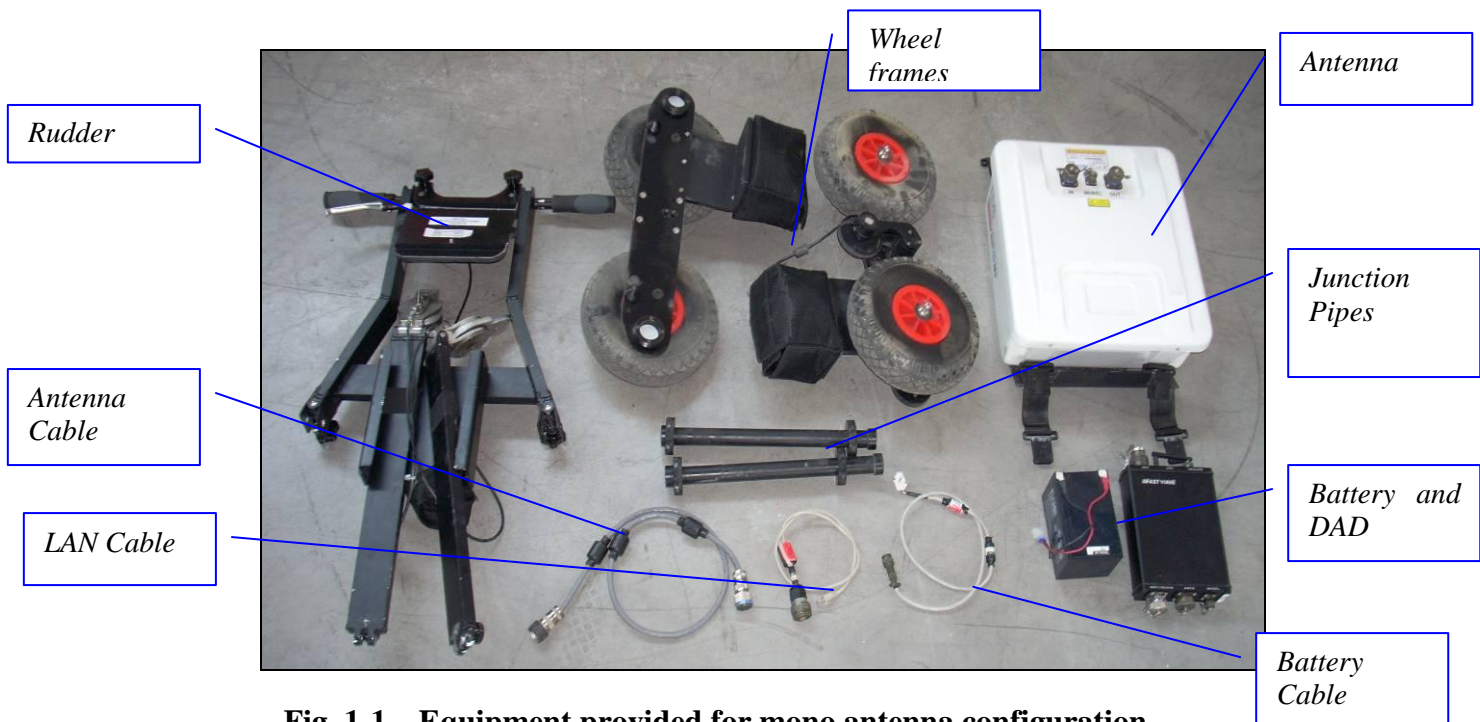
Fig. 1-1 – Equipment provided for mono antenna configuration
