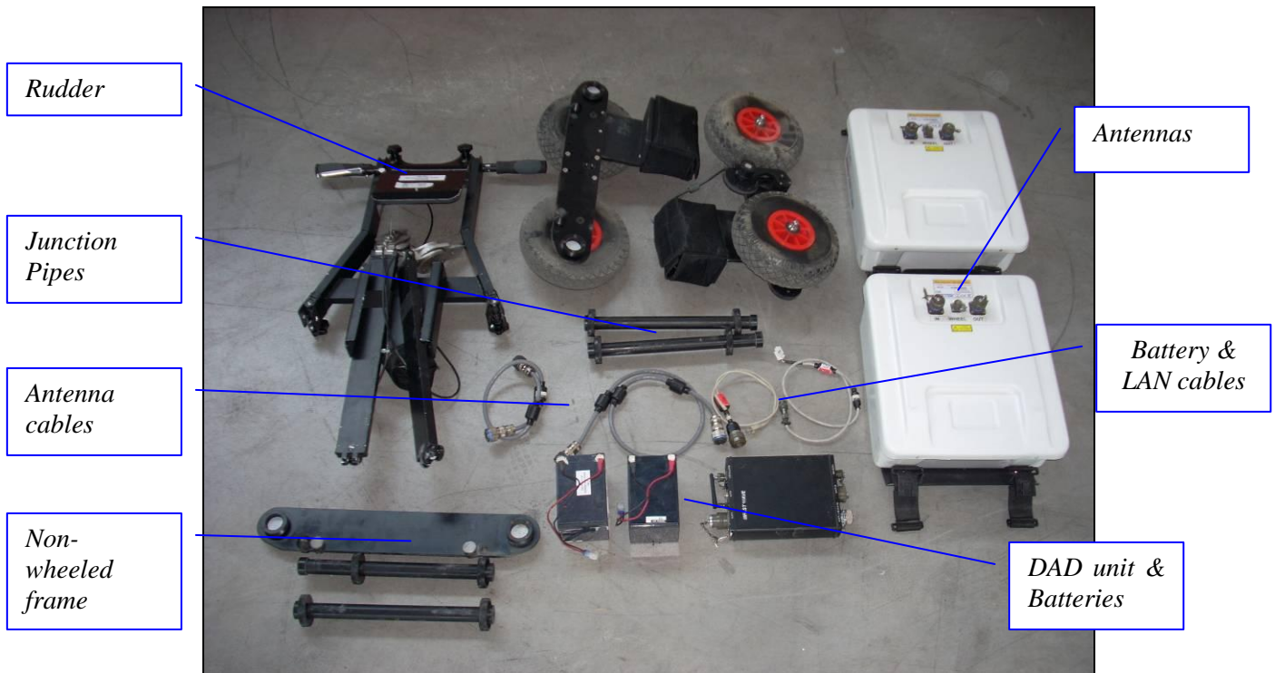
Fig. 1-13 – Equipment provided for the two antennas configuration
