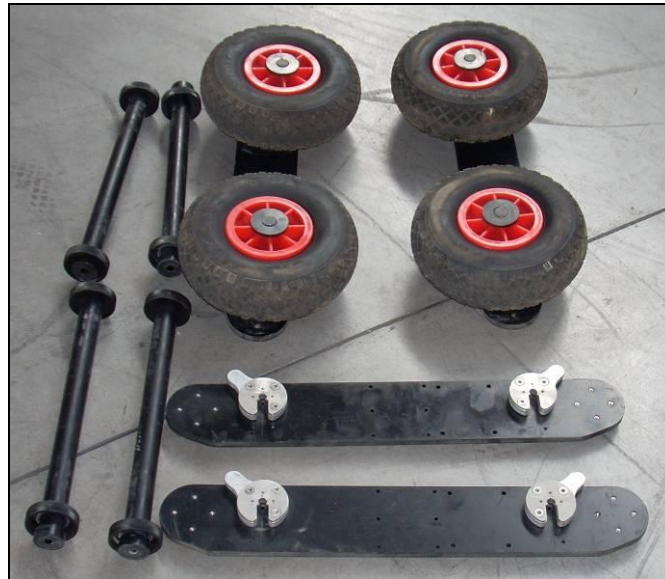
Fig. 1-22 – Side antenna frames parts
