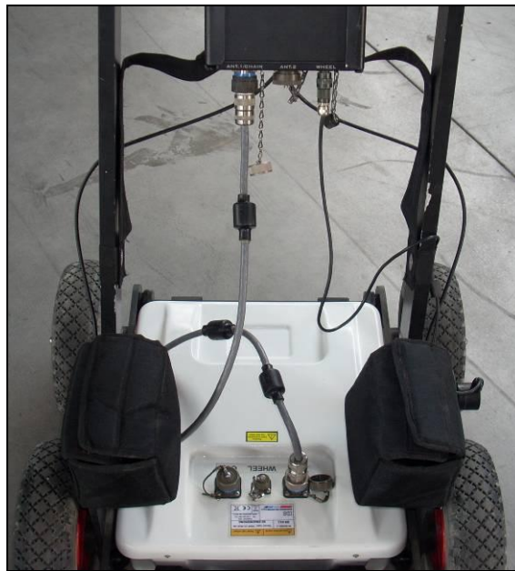
Fig. 1-11 – Antenna cable in place
