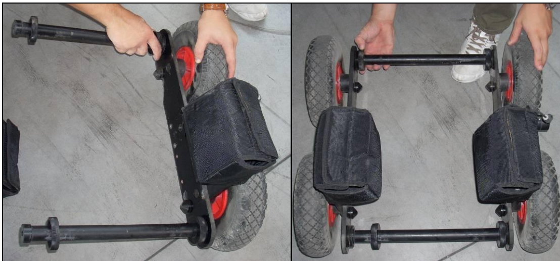
Fig. 1-5 – Junction pipes in position and closed frame
