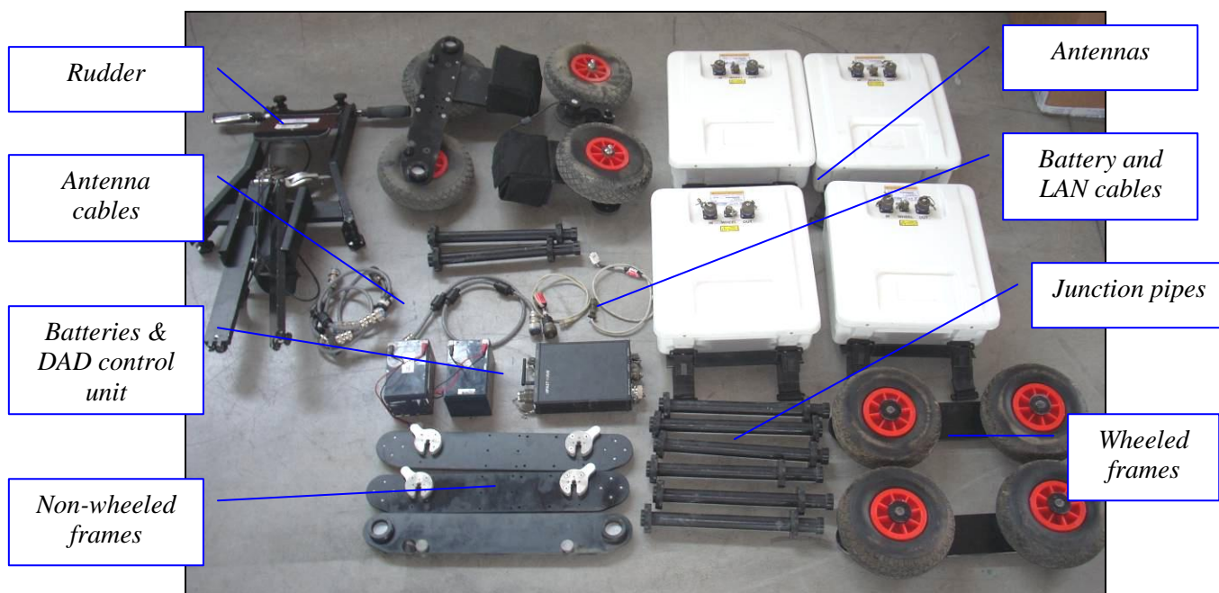
Fig. 1-28 - Equipment provided for the four antennas configuration
