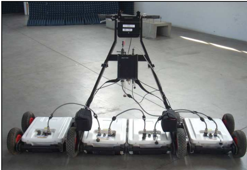
Fig. 1-30 – Four antennas configuration
