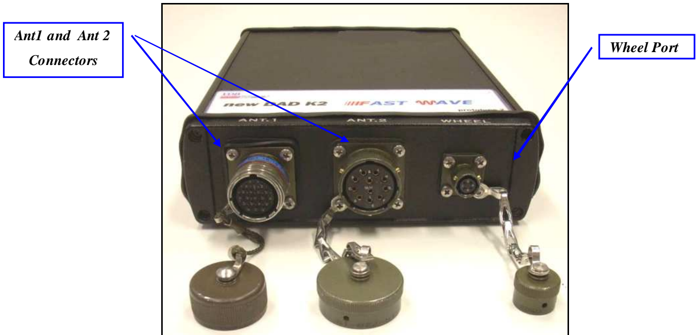
Fig. 2-2 – –DAD side Fast Wave with connections to position sensor and antennae
