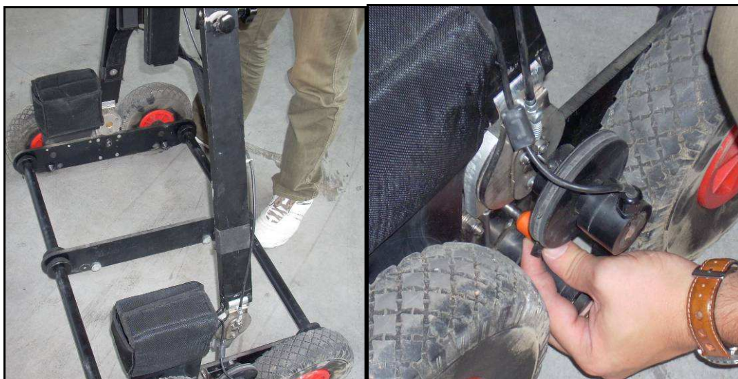
Fig. 1-17 – Insertion and locking of the rudder
