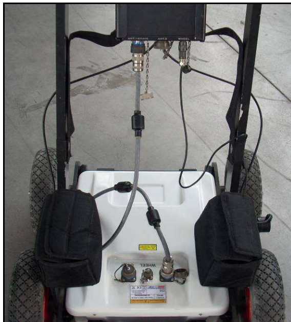
Fig. 1-11 – Antenna cable in place
