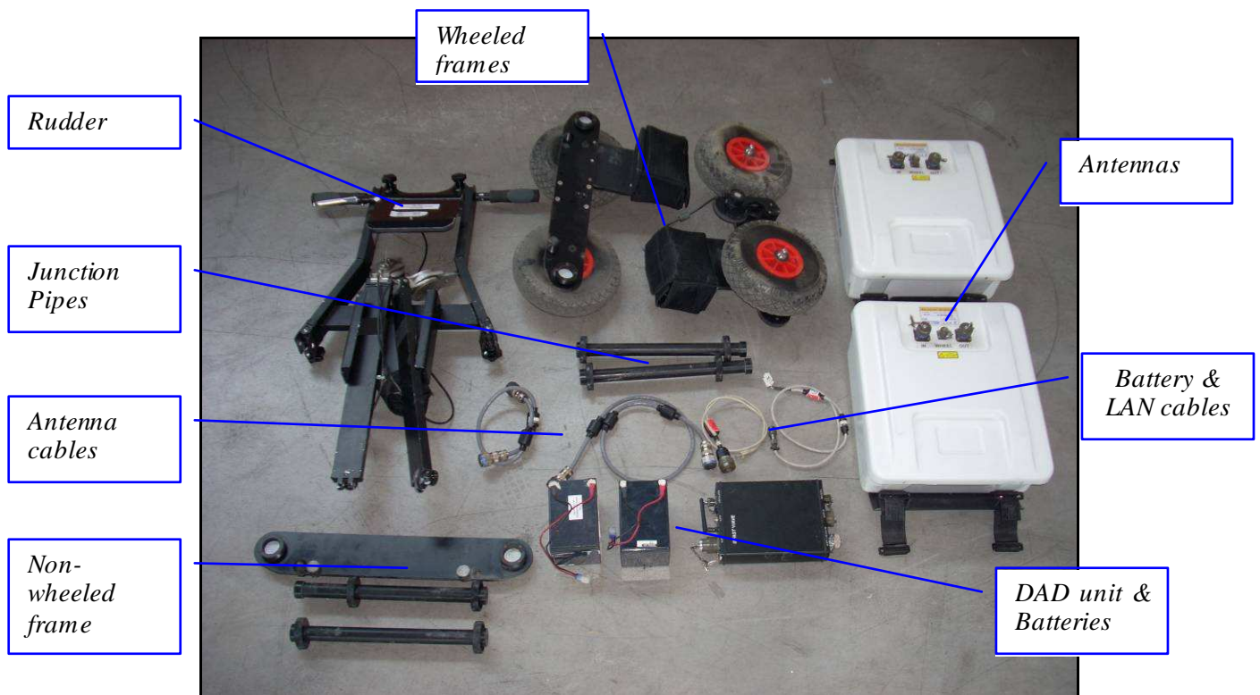
Fig. 1-13 – Equipment provided for the two antennas configuration
