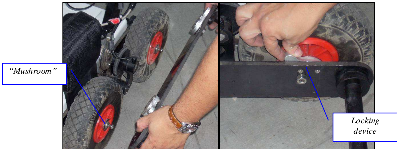
Fig. 1-24 – Main frame “mushrooms” & locking device
