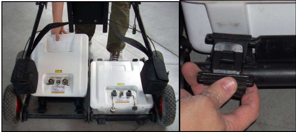
Fig. 1-18 – Insertion of the antennas and close-up of the hook
