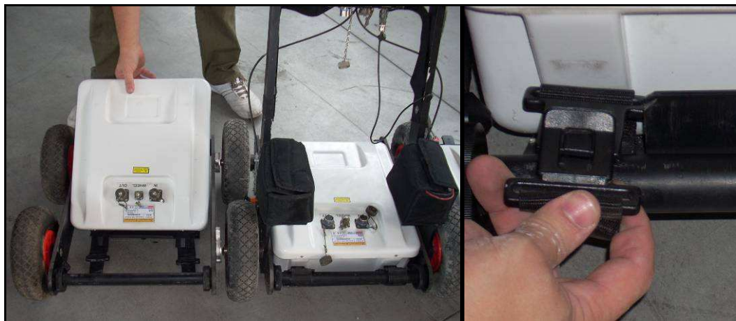
Fig. 1-25 - Insertion of one antenna and close-up of the hook
