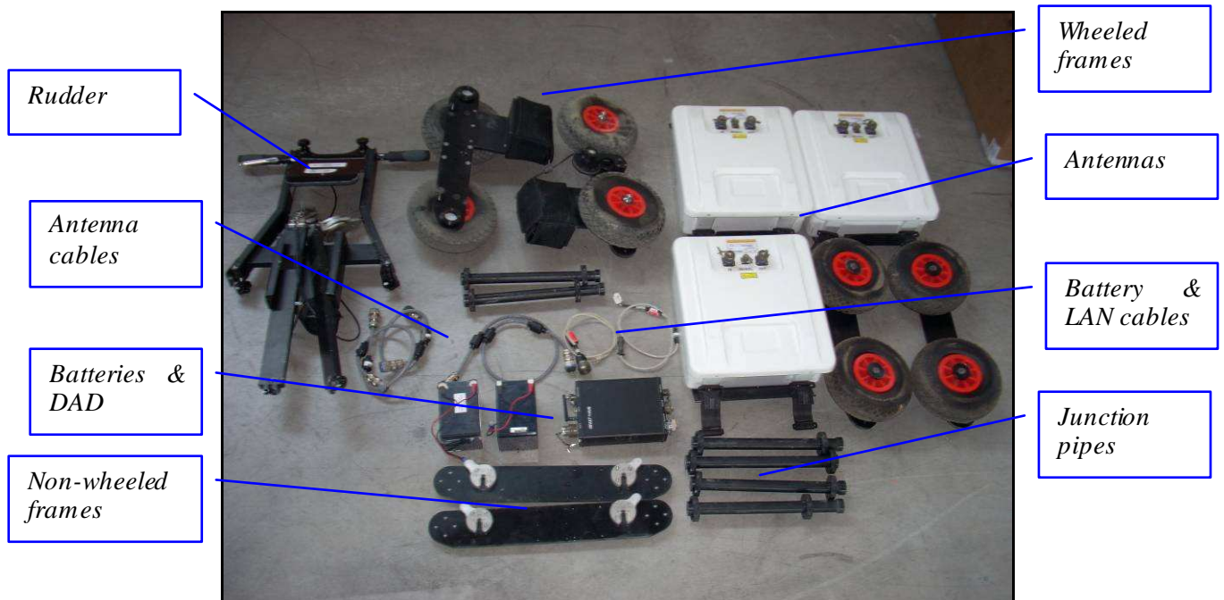
Fig. 1-21 - Equipment provided for the three antennas configuration
