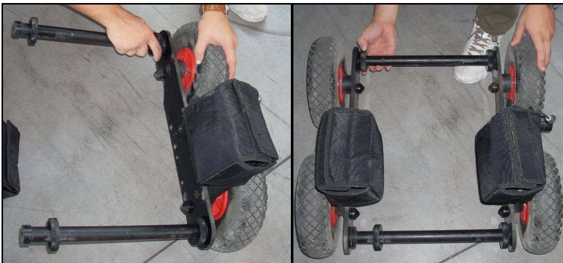
Fig. 1-5 – Junction pipes in position and closed frame
