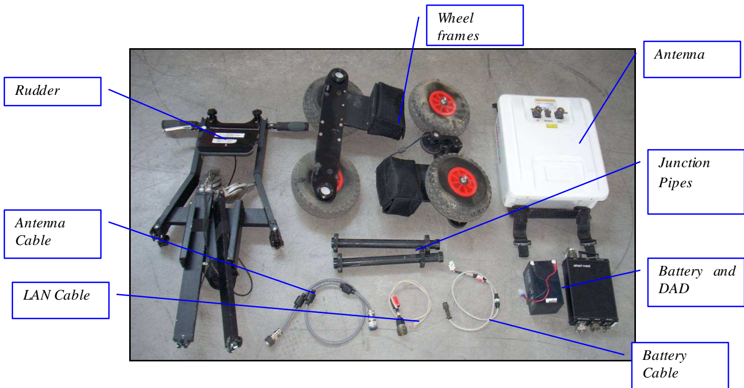
Fig. 1-1 – Equipment provided for mono antenna configuration
