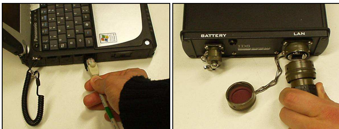
Fig. 2-7 – Lan Cable connection between the Notebook Computer and the DAD Control Unit
