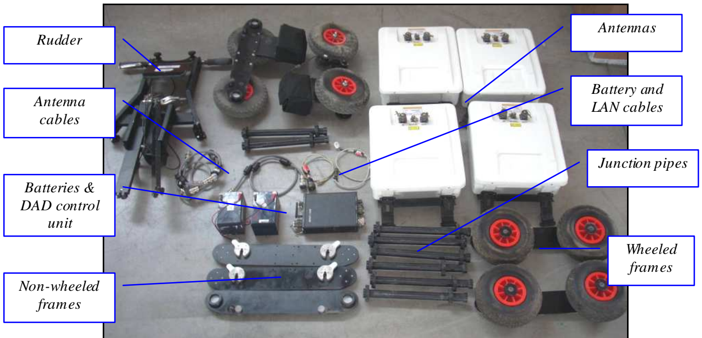
Fig. 1-28 - Equipment provided for the four antennas configuration
