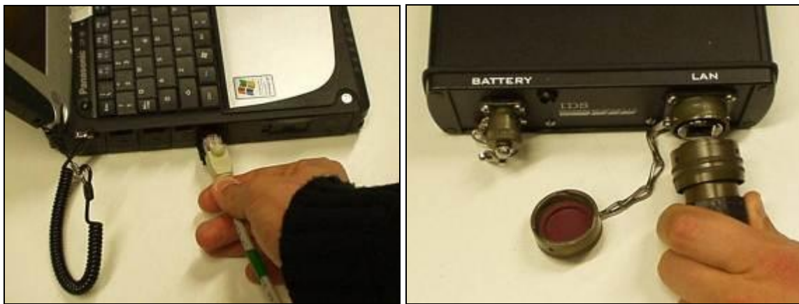
Fig. 5.3 – Lan Cable connection between the Notebook Computer and the DAD Control Unit
