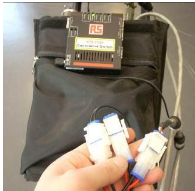
Fig. 3.4 – Ethernet switch power supply cable
