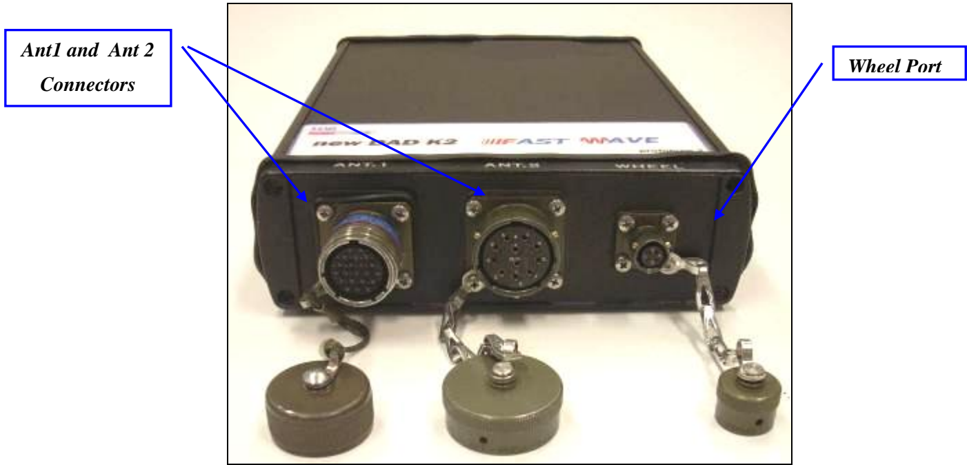
Fig. 4.2 – –DAD side Fast Wave with connections to position sensor and antennae
