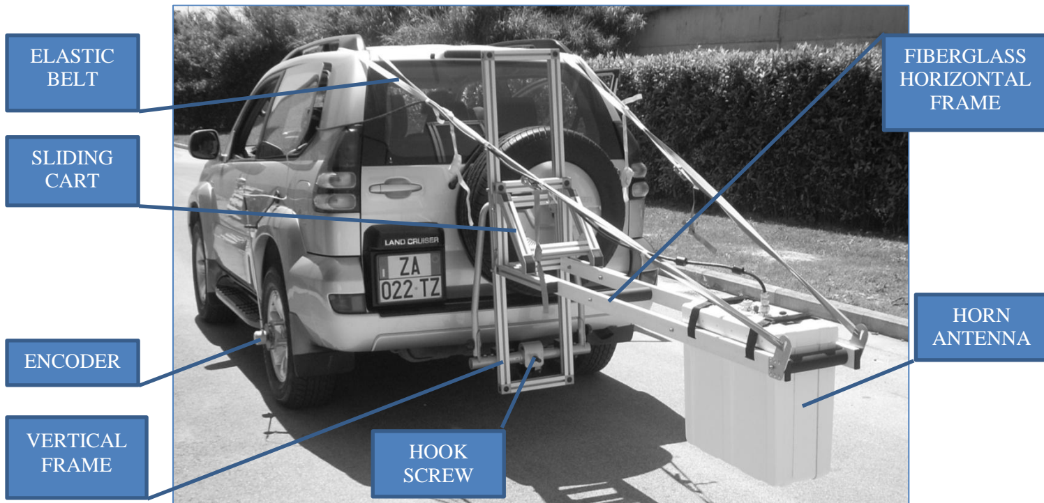
Fig. 1-1– Composition of the Hi-Pave system
