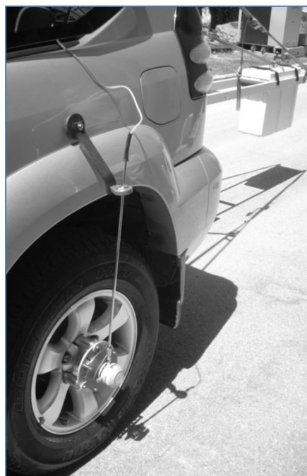
Fig. 2-10 – Encoder wheel kit view
