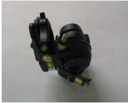
Fig. 5.20 – Position of the body of the three axial head when packing it away
