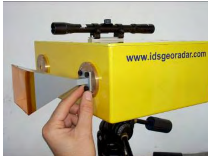
Fig. 5.13 – Mounting the antennas
