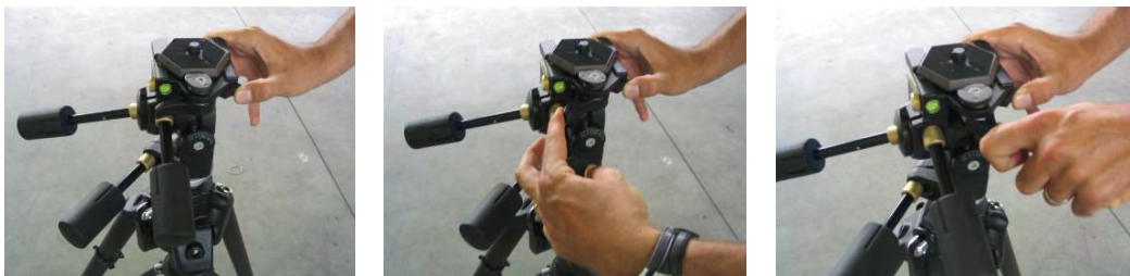
Fig. 5.8 – Unlocking the levers of the quick lock mechanism
