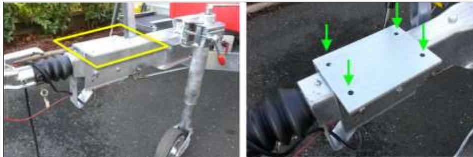
Fig. 81 – Plate installed on the front part of the trailer shaft
