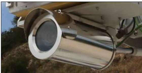
Fig. 14 – Camera fixed below the sensor trolley
