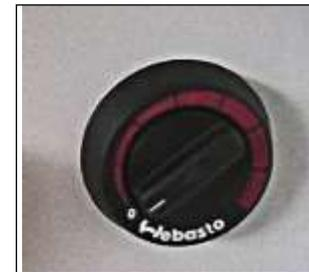
Fig. 40 – Webasto® Heater temperature control
