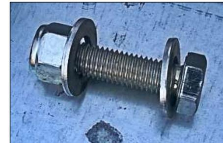
Fig. 43 - M12 x 50 mm hexagonal head screw with self-blocking nut and washer
