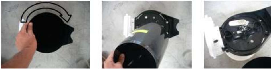
**Fig. 63 – Remove the rain gauge funnel**
