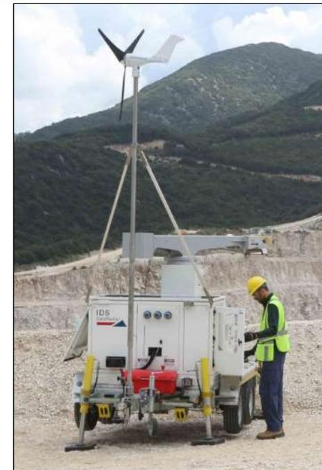
Fig. 93 – Wind turbine and pole installed on IBIS ArcSAR
