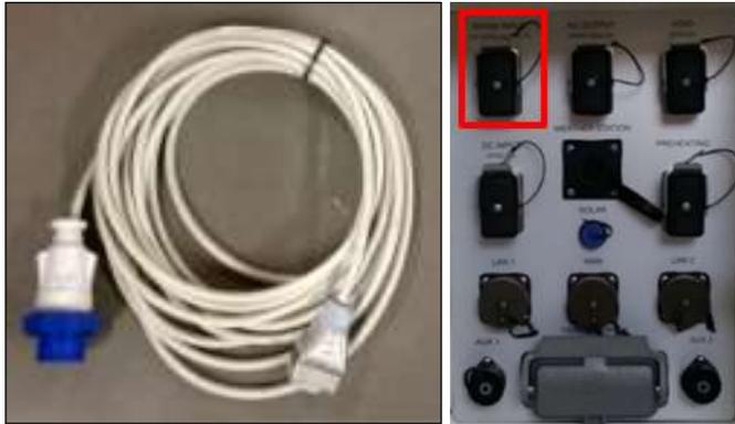
Fig. 148 – Connections to supply IBIS-ArcSAR with AC Mains power
