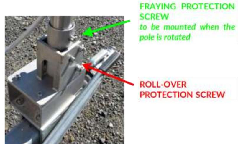
Fig. 82 – Pole metallic base installed on the trailer shaft
