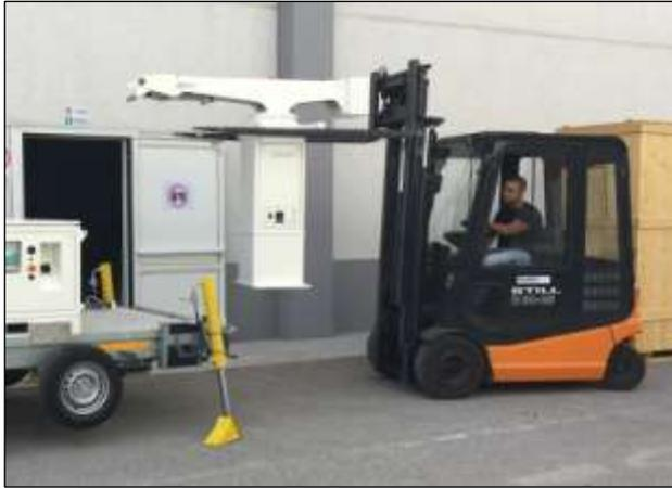
**Fig. 51 – Lifting the Acquisition Unit with the forklift**
