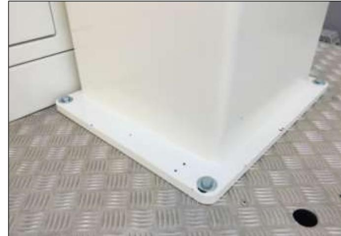
**Fig. 53 – Fix the Acquisition Unit base to the trailer**
