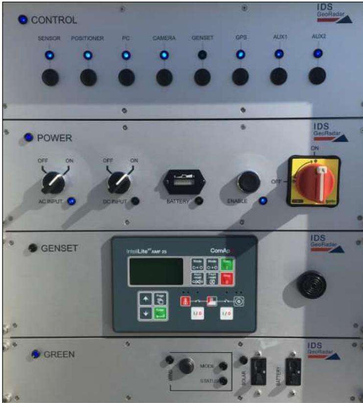
**Fig. 13 – Modules on the front side of PSU**
