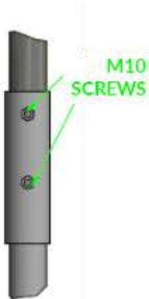
Fig. 85 – Metallic pole joint
