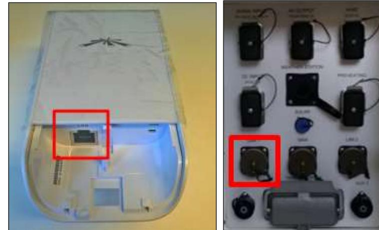
Fig. 70 – Wi-Fi sockets in the radio and in the rear I/O interface panel
