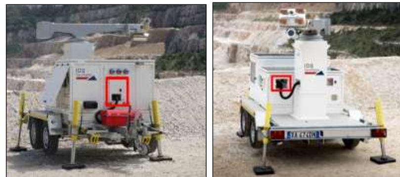
Fig. 18Figure 1 – Positions of the I/O interfaces panels on IBIS-ArcSAR
