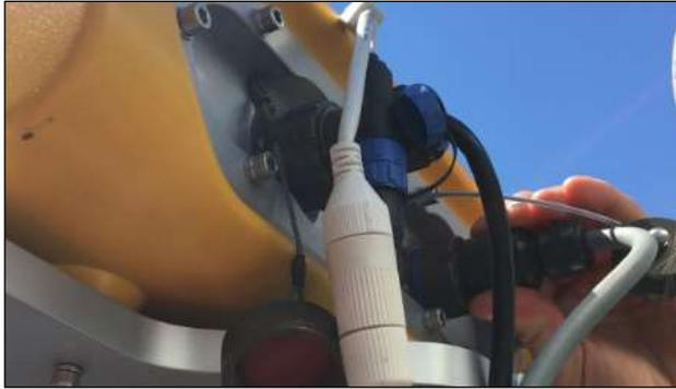
Fig. 97 – ETHERNET and SUPPLY connections to the Sensor
