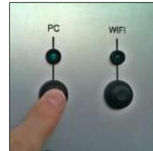
Fig. 154 – PC Switch on Control Module
