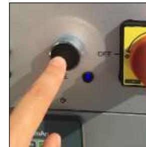
Fig. 147 – Turning on the ENABLE switch in the Power Module on PSU panel
