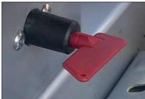
Fig. 135 – Hydraulic system battery cut-off switch
