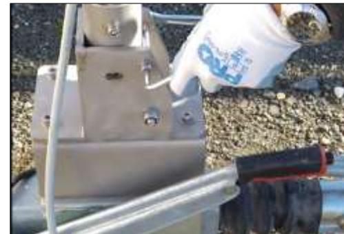
Fig. 83 - Remove the roll-over protection screw
