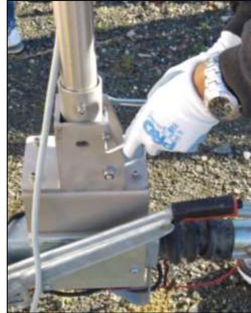
**Fig. 91 – Pole tightened to the trailer**
