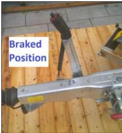
Fig. 130 – Pulling hand brake
