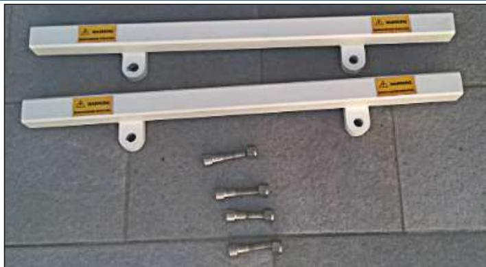
Fig. 55 - Wings removed from the Acquisition Unit
