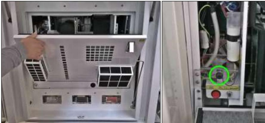
Fig. 106 – Fuel filter cleaning
