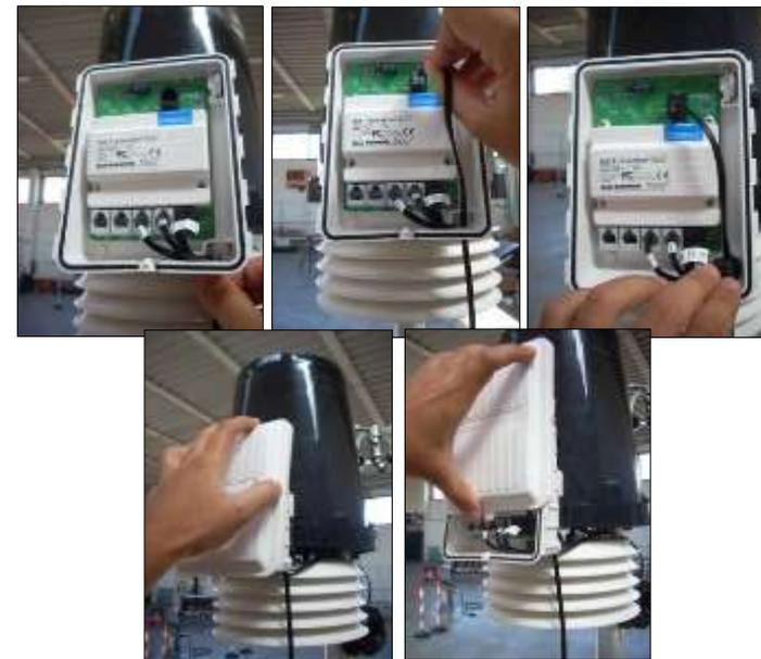
Fig. 67 – Weather Station cable connections (3/6)
