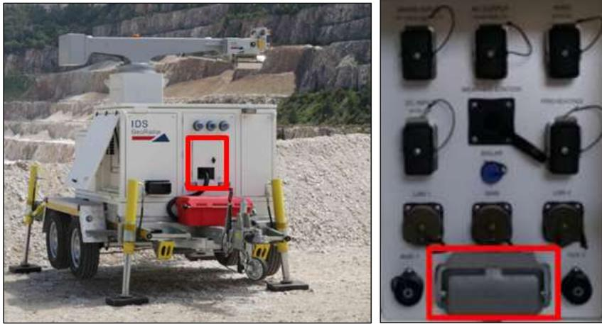
Fig. 94 – I/O Interfaces panel containing the Trailer Supply socket
