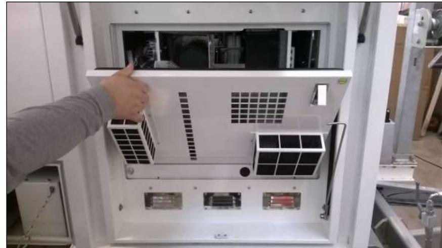
Fig. 101 – Opening the Generator internal panel
