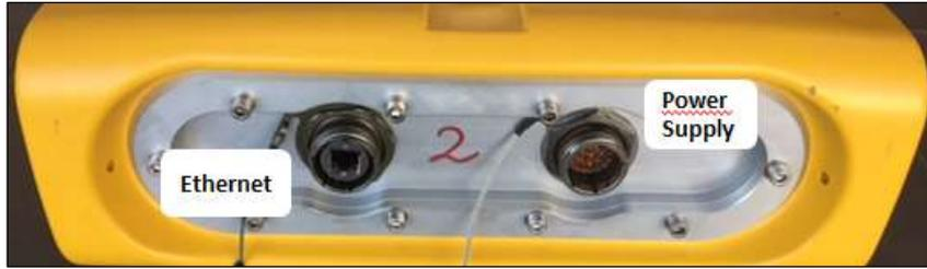
Fig. 5 – Back view of the Radar Sensor
