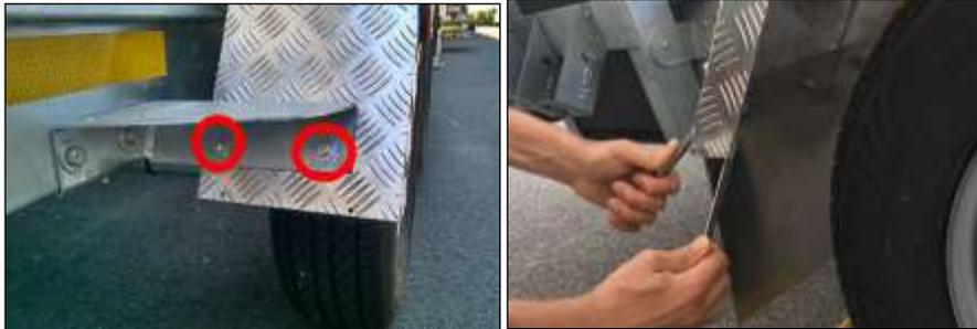
Fig. 44 – Mudguards fixing screws
