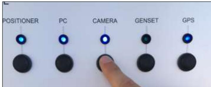
Fig. 152 – Turning the CAMERA switch on (PSU Control module)
