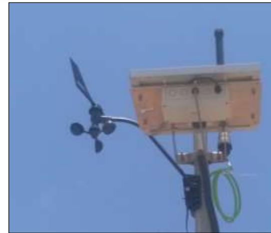
Fig. 75 – Genset solar panel installed on the pole
