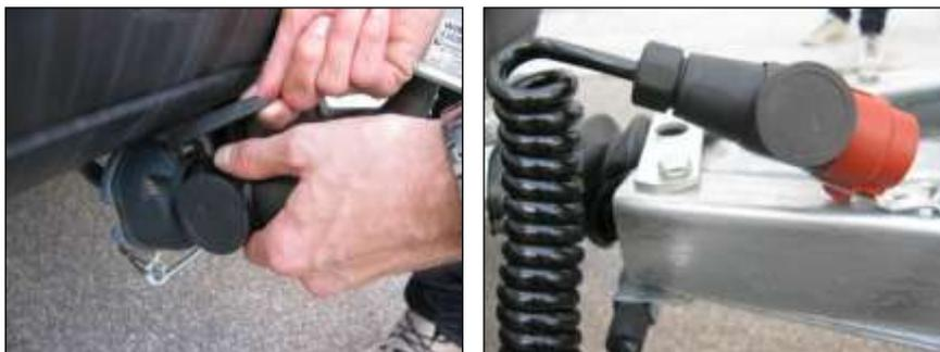
Fig. 131 – Disconnecting trailer cable
