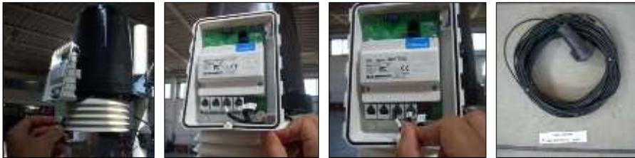
Fig. 66 – Weather Station cable connections (2/6)
