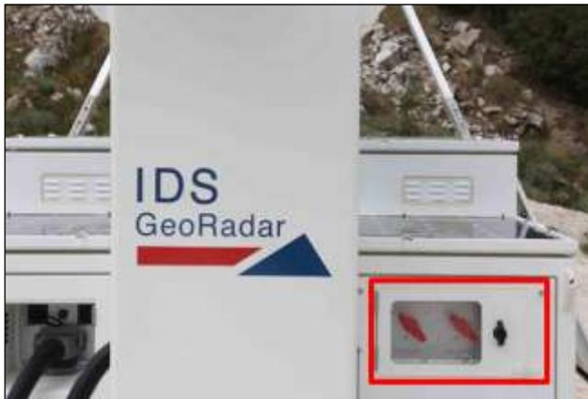
Fig. 138 – Isolation Point panel on Supply Unit front side
