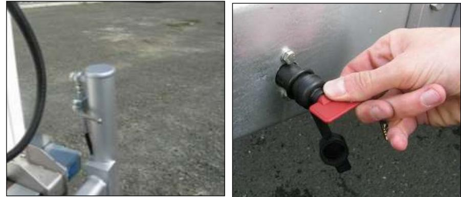
**Fig. 142 – Secure the jacks**
