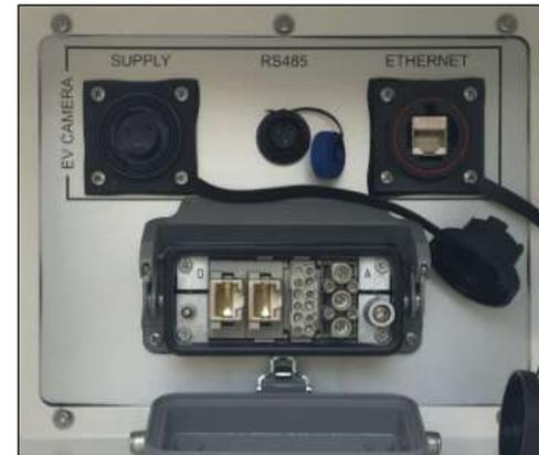
**Fig. 20 – Interface panel on the front side of the ArcSAR Supply Unit**
