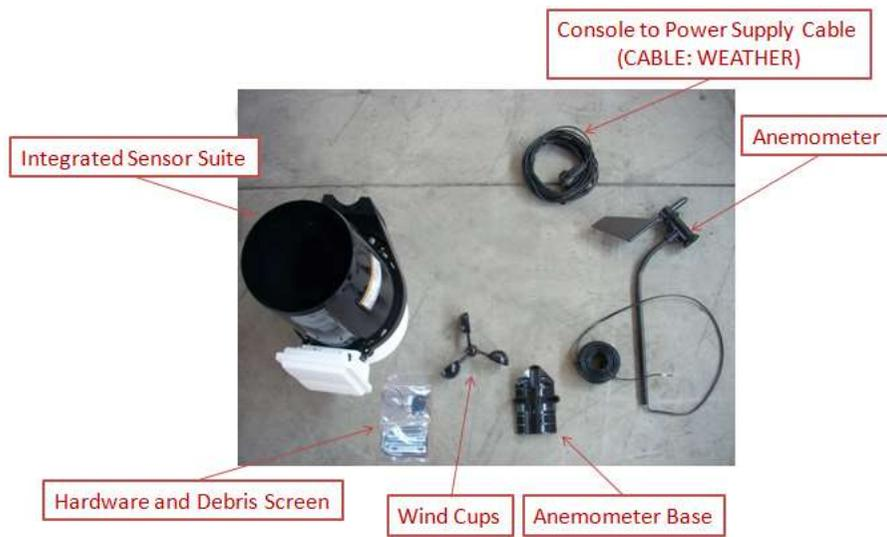
Fig. 35– Components of the Weather Station
