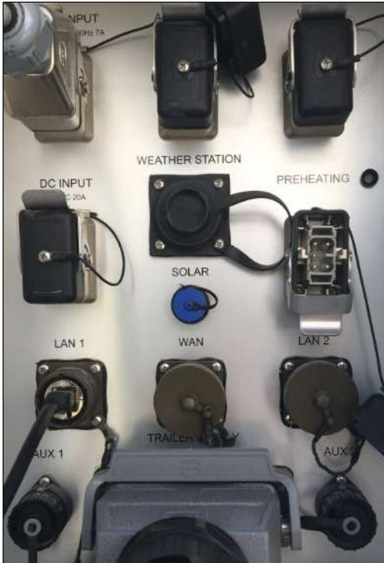
**Fig. 19 – Interface panel on the rear side of the IBIS-ArcSAR Supply Unit**
