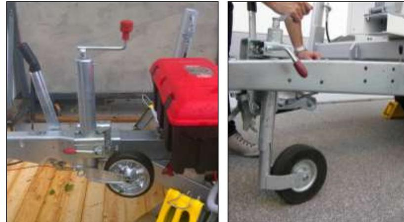
Fig. 132 – Lowering the front wheel of the cart
