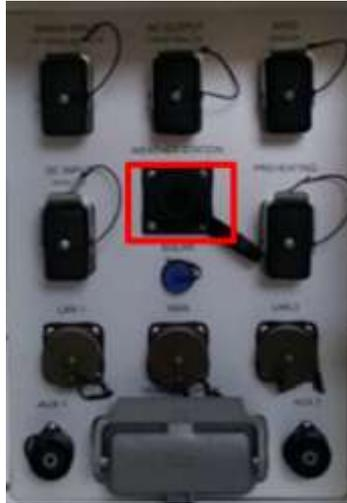
Fig. 68 – Weather Station connection on the I/O interface right panel
