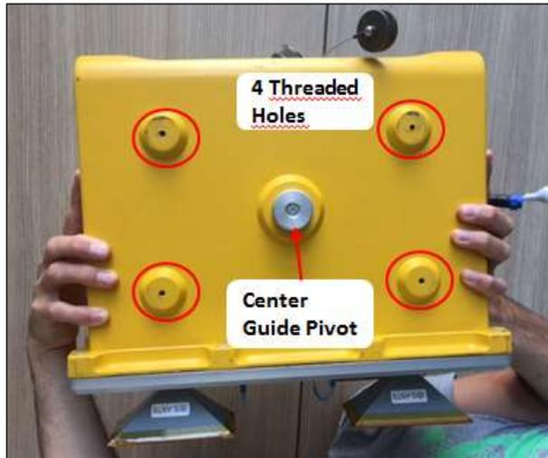
Fig. 6 – Bottom view of the Radar Sensor
