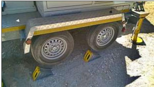
**Fig. 141 – Right trailer horizontal levelling**
