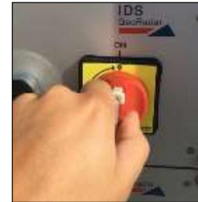
Fig. 146 – Turning on the PSU ON/OFF switch
