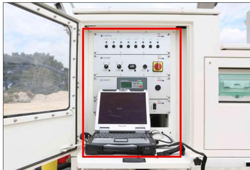
Fig. 12 – Power Supply Unit position on the left side of the IBIS-ArcSAR
