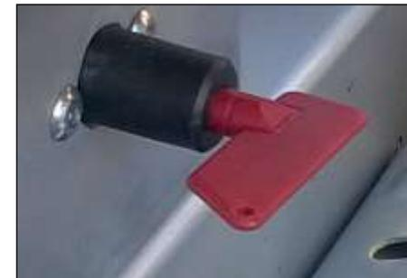
**Fig. 28 – Battery cut-off switch**
