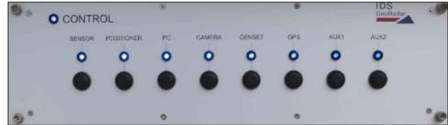
**Fig. 14 – Front side of the Control module**
