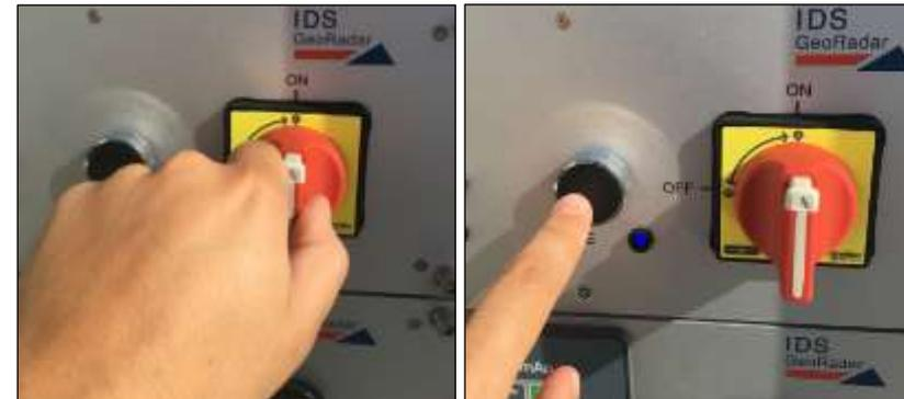
Fig. 108 – Turning on the system
