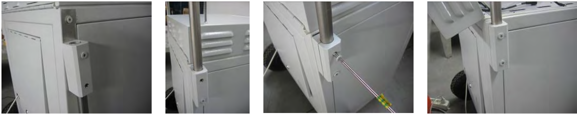
Fig. 3.21 - Sequence for unfolding the power supply unit handles
