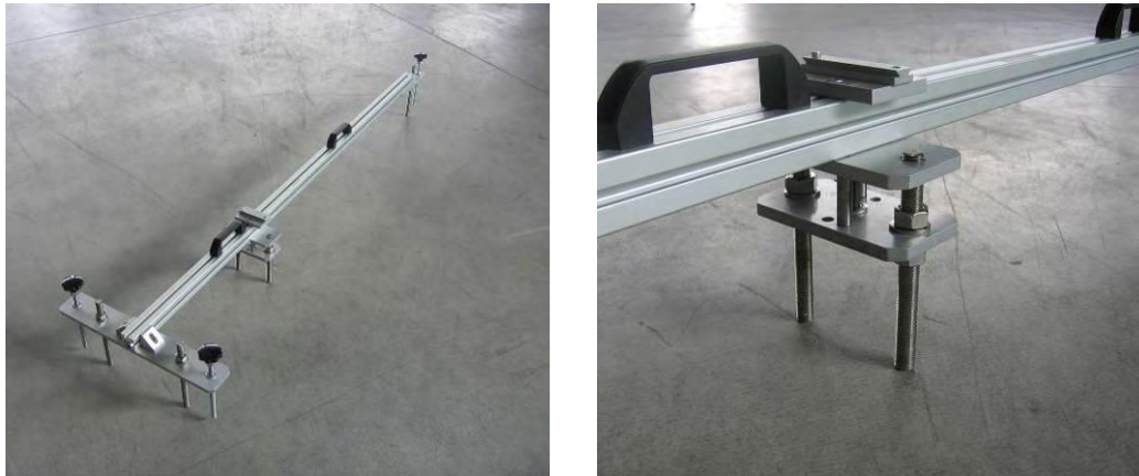
Fig. 4.9 – Mounting the studs on the template, detail of the central plate with the spacer and its two studs
