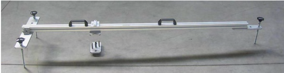
Fig. 3.18 – View of the drilling and positioning template with spacer
