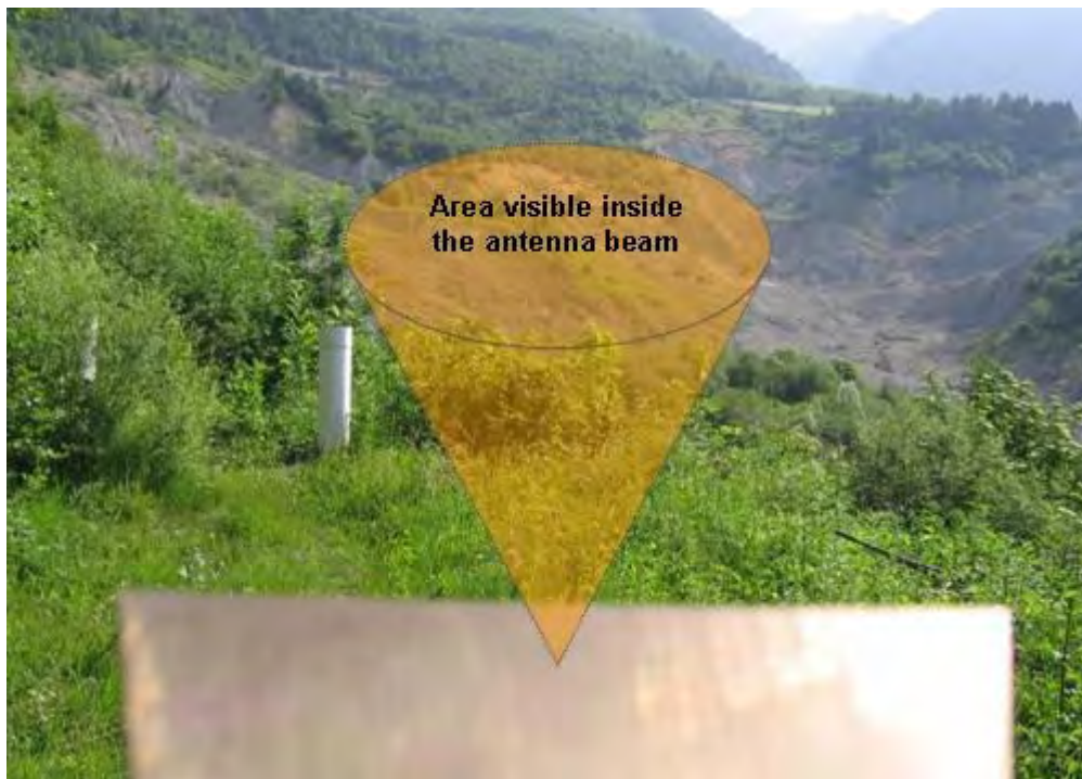
Fig. B. 2 – Area of the scenario covered by the antenna beam main lobe.
