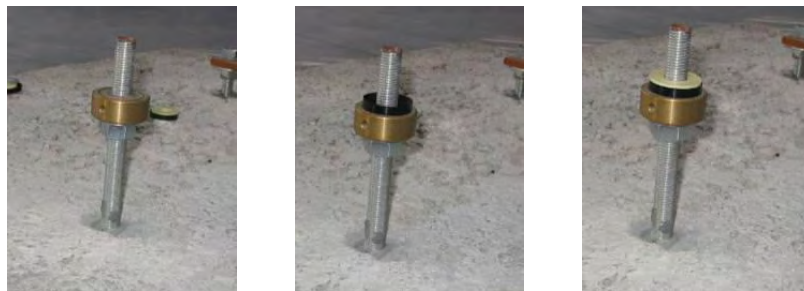
Fig. 4.13 – Sequence for mounting the spherical thrust bearings
