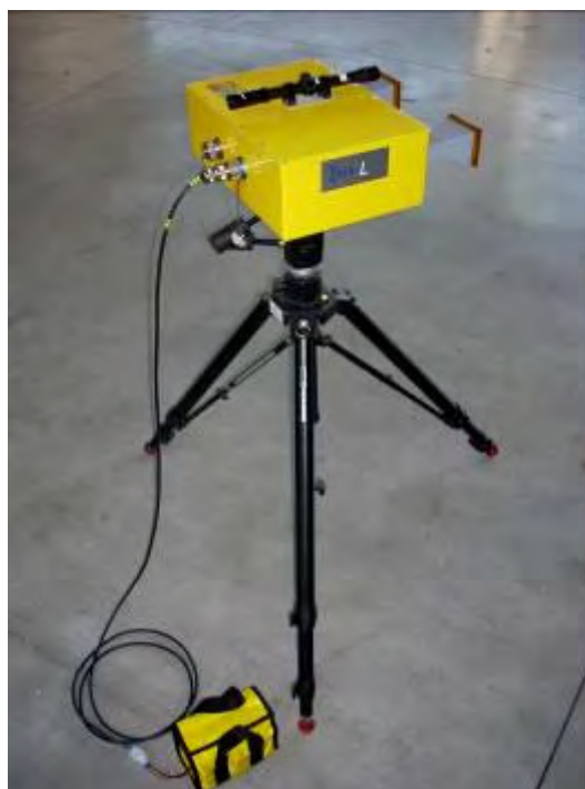
Fig. 5.16 – Connecting the sensor to the battery
