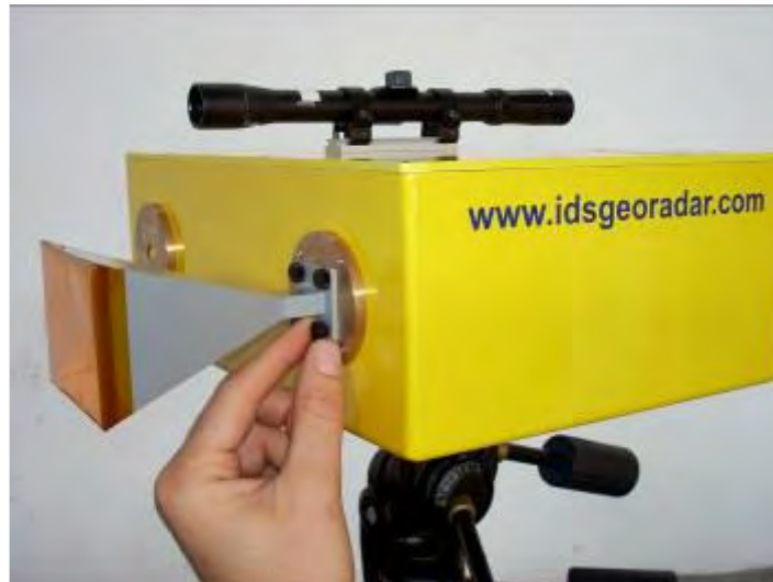
Fig. 5.13 – Mounting the antennas
