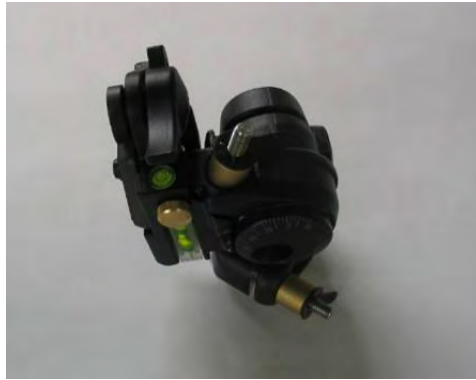
Fig. 5.20 – Position of the body of the three axial head when packing it away
