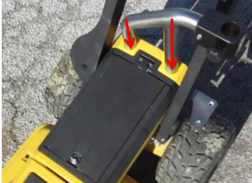
Fig. 4.14 – GPS support upper part insertion
