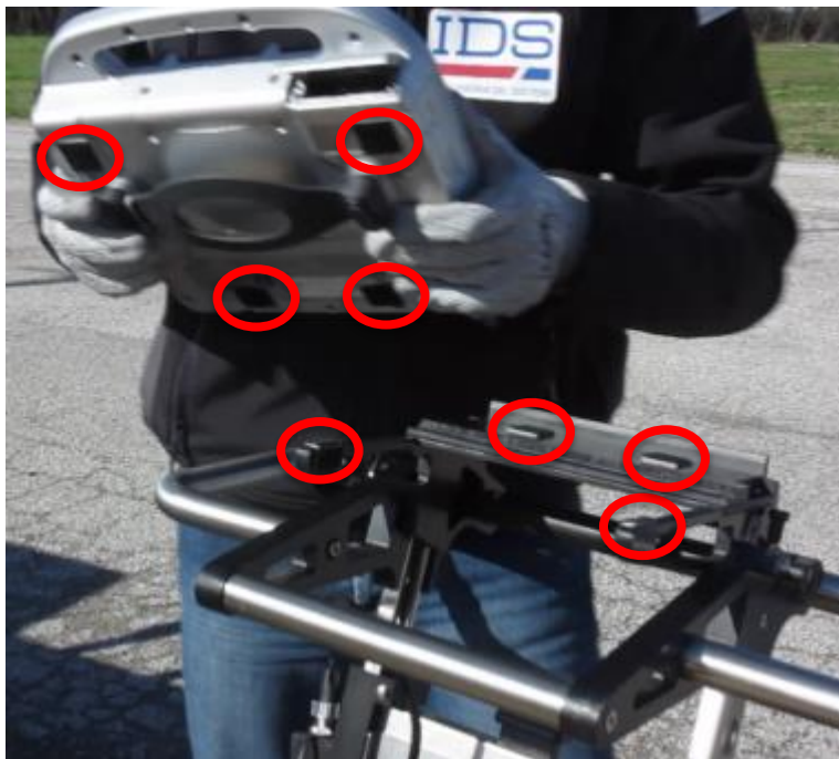
Fig. 4.6 – Velcro strips on the Laptop and Laptop support
