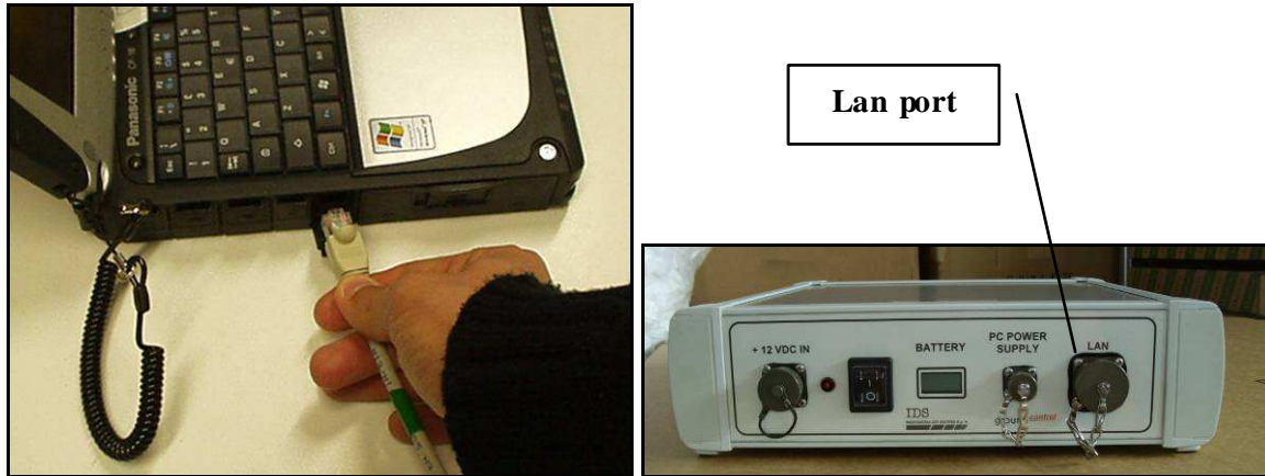
Fig. 2-8 – Lan Cable connection between the Notebook Computer and the Control Unit (SRS_PLUS)
