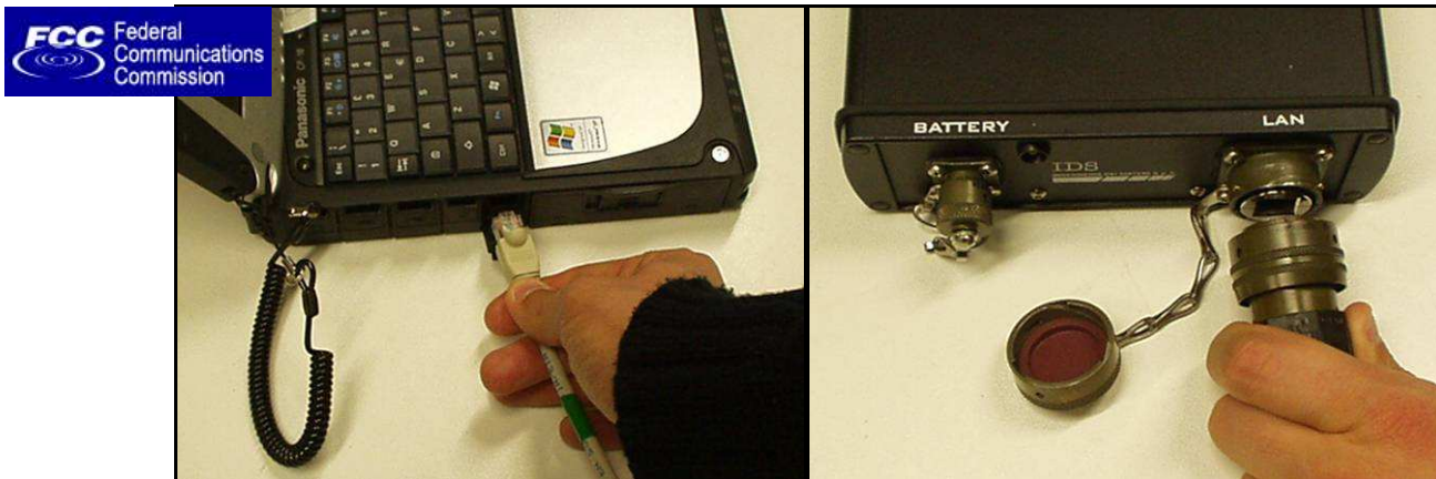
Fig. 2-9 – Lan Cable connection between the Notebook Computer and the Control Unit (SRS-FW400 only)
