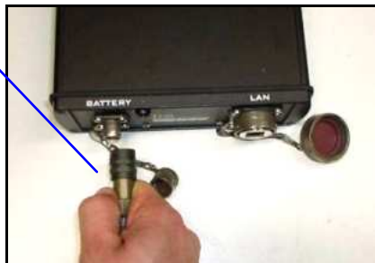
Fig. 2-13 – Connecting the Control Unit to the battery (SRS-FW400 only)
