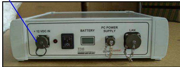
Fig. 2-11 – Connecting the Control Unit to the battery (SRS_PLUS)
