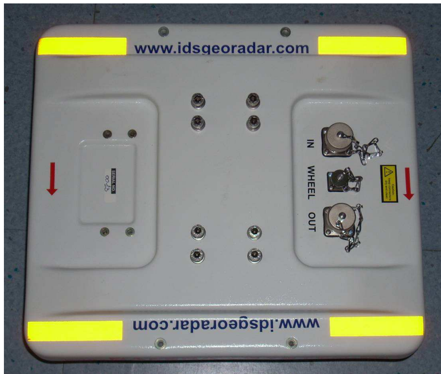
Fig. 2-19 –Antenna for the SRS-FW400 system (red arrows show dragging direction)
