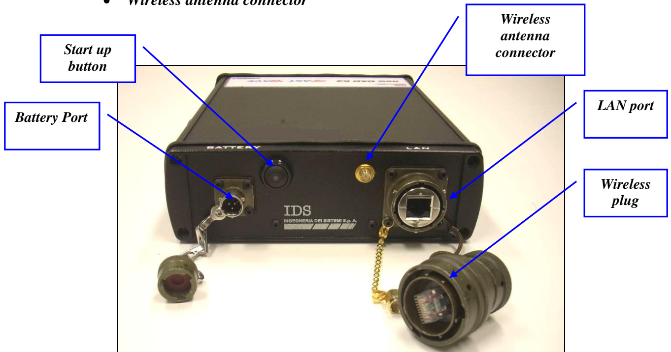
Fig. 1.8 – DAD side Fast Wave with Battery Port, Lan Port and wireless connector
