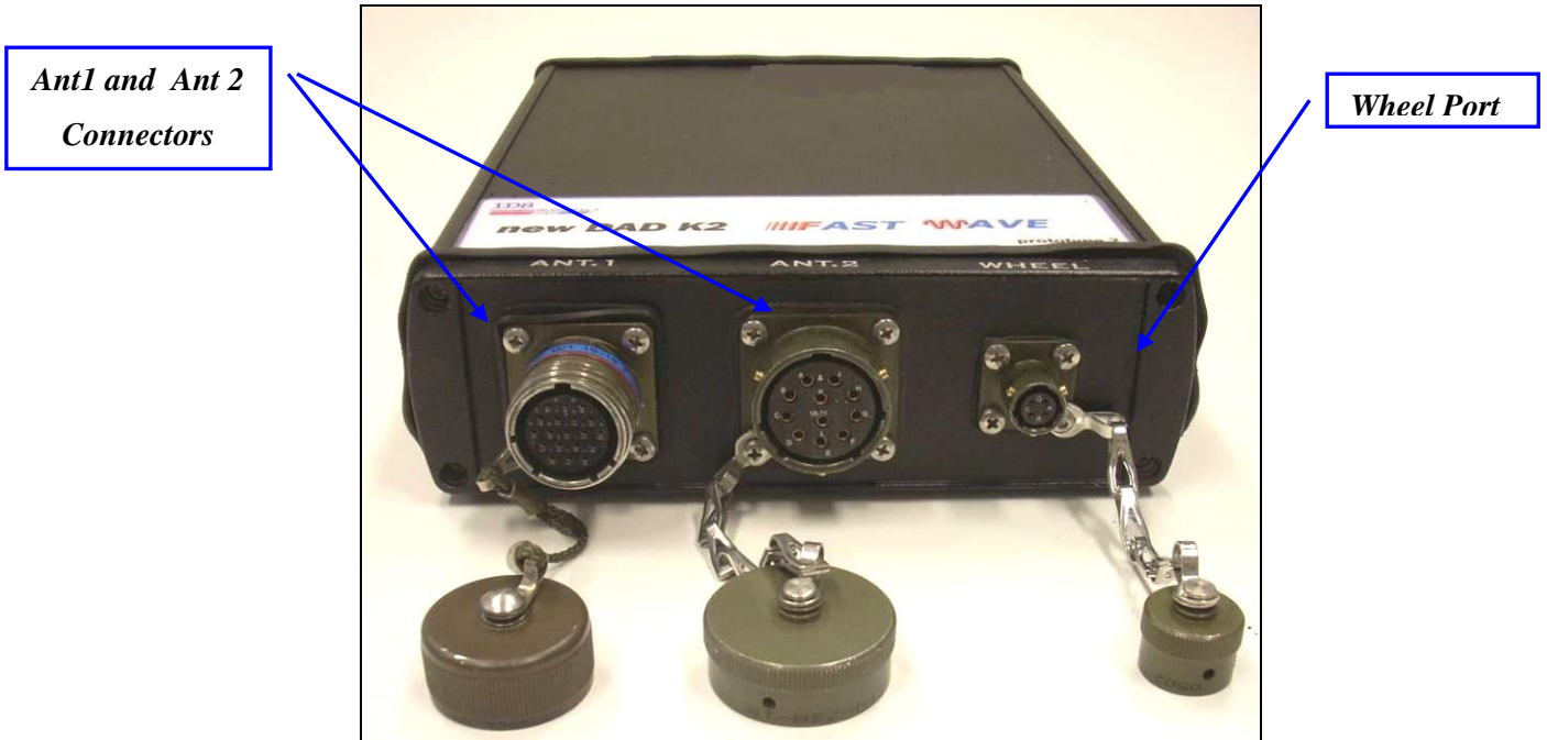
Fig. 1.9 – –DAD side Fast Wave with connections to position sensor and antennae
