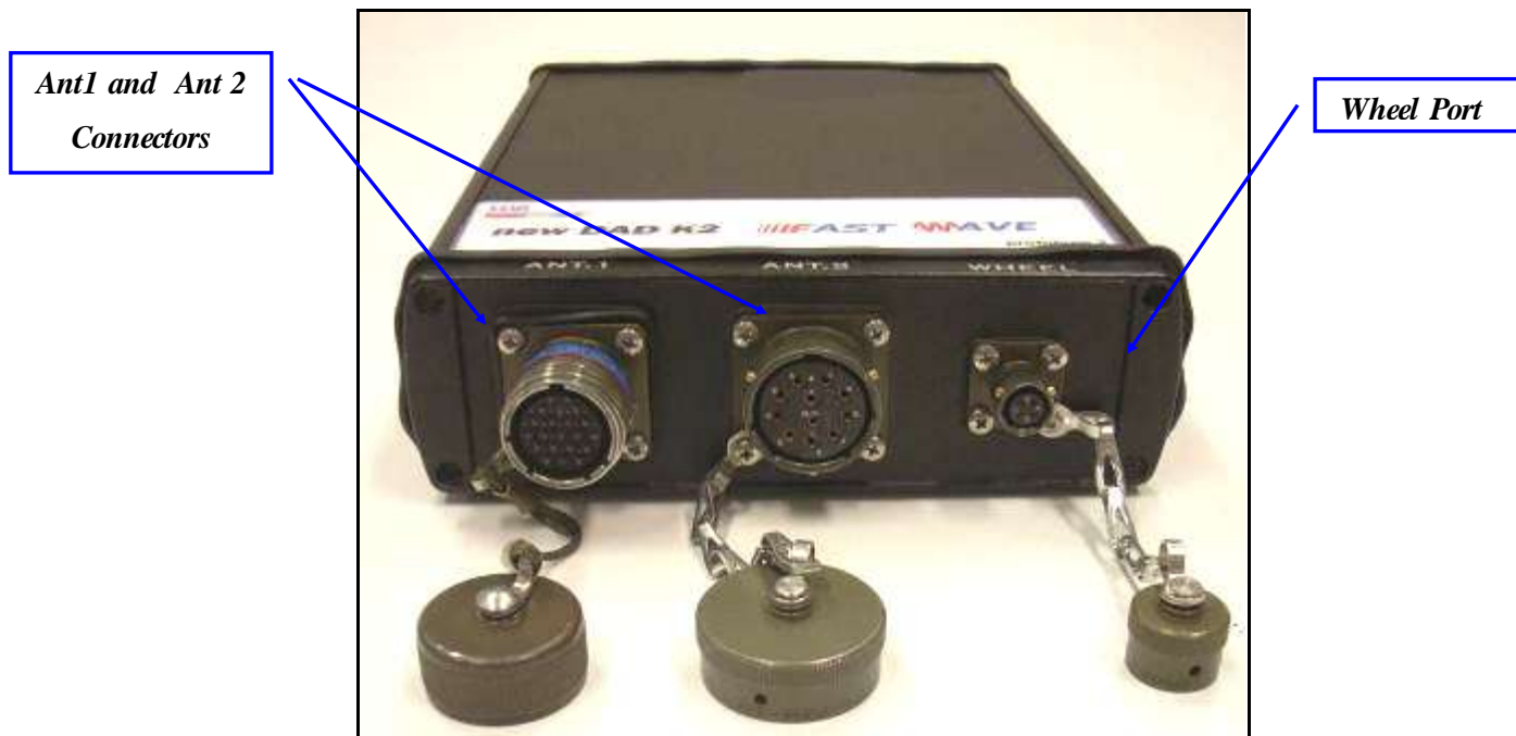
Fig. 4.2 – DAD side Fast Wave with connections to position sensor and antennae
