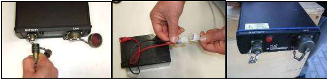
Fig. 5.5 – Connecting the DAD Control Unit to the battery pack and switching on button (red color)
