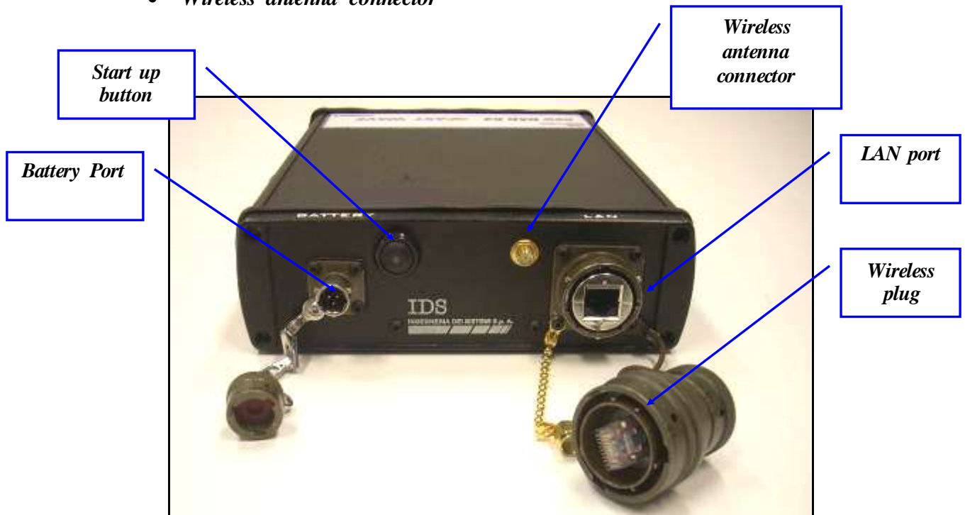
Fig. 4.1 – DAD side Fast Wave with Battery Port, Lan Port and wireless connector
