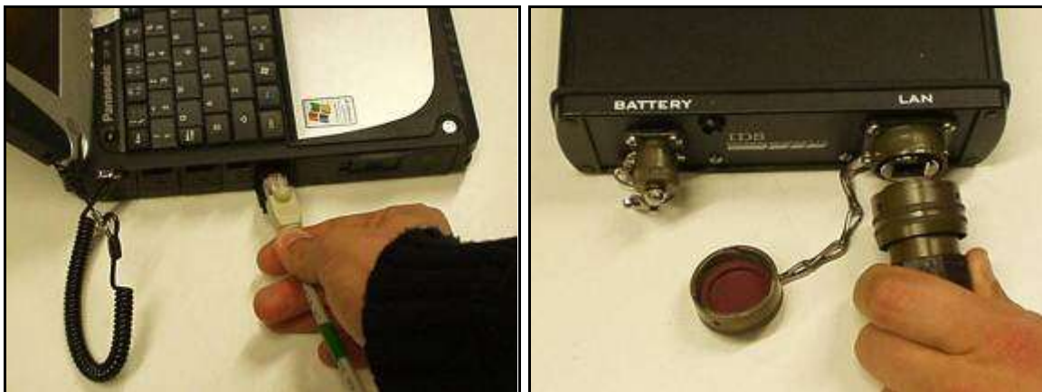
Fig. 5.3 – Lan Cable connection between the Notebook Computer and the DAD Control Unit
