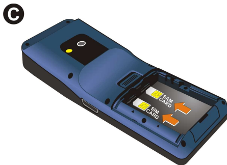
Figure 2-6: Inserting the SIM/SAM Card
