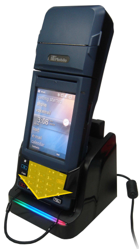
Figure 2-3: Connect the MODAT-100 to the Charging Cradle
