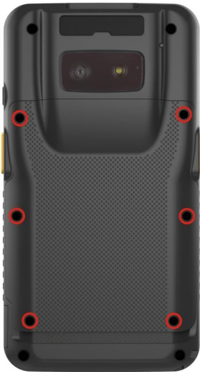
Figure 3-4: Battery Cover Retention Screws
