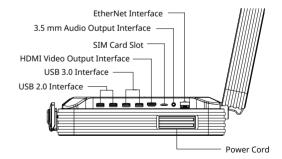
**Note:** SIM Card Slot is compatible with China Mobile and China Unicom.
