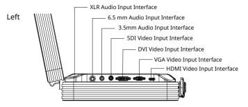
**Note:** HDMI cable featuring magnetic ring and shield is suggested when connecting HDMI interface.
