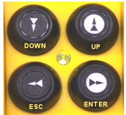
Figure 9 Pushbutton as a Key board for Hoist Condition Monitoring Unit
